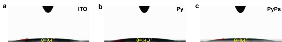
Fig. S23. Contact angles of perovskite precursor solution on (a) ITO, (b) Py and (c) PyPs substrates.
