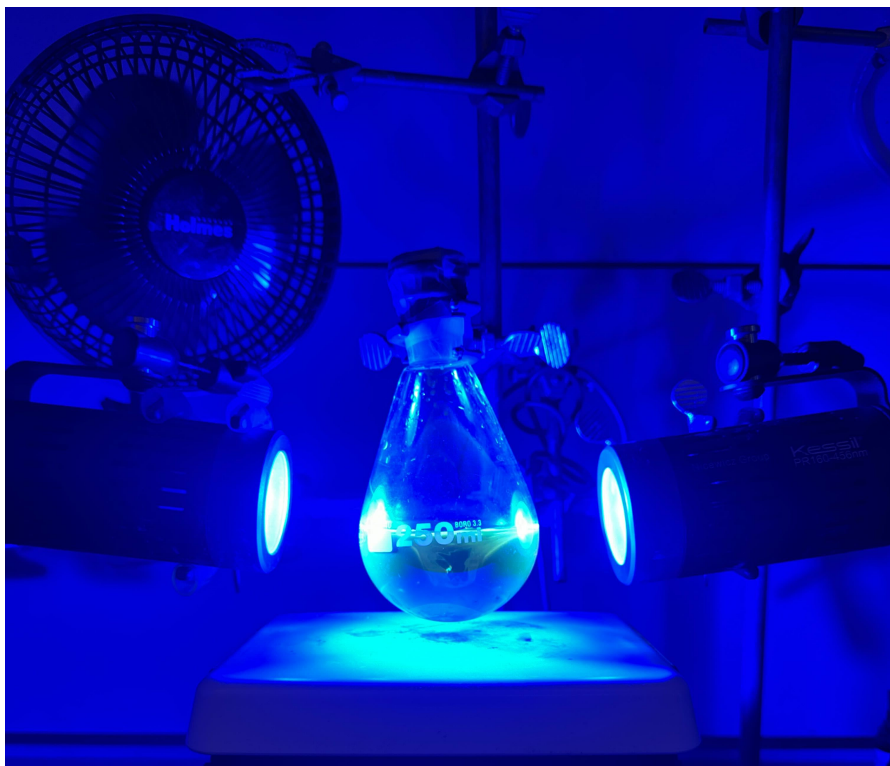
Figure S6 Batch reaction setup highlighting the placement of the 456 nm Kessil lamps, stir plate, and fan. Not pictured is a protective shield to contain the irradiation.
