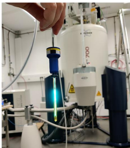
Figure S49. NMR sample with quartz glass insert and optical fibre for in-situ illumination during NMR experiments.
