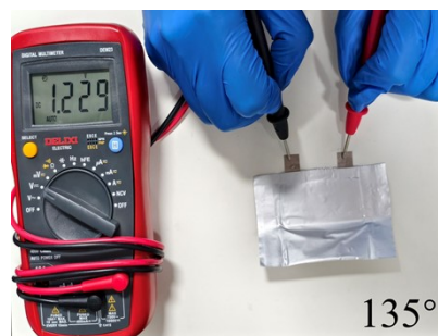
Fig. S20. The open circuit voltage of TNVO@GO soft pack battery at 135^\circ bending states.
