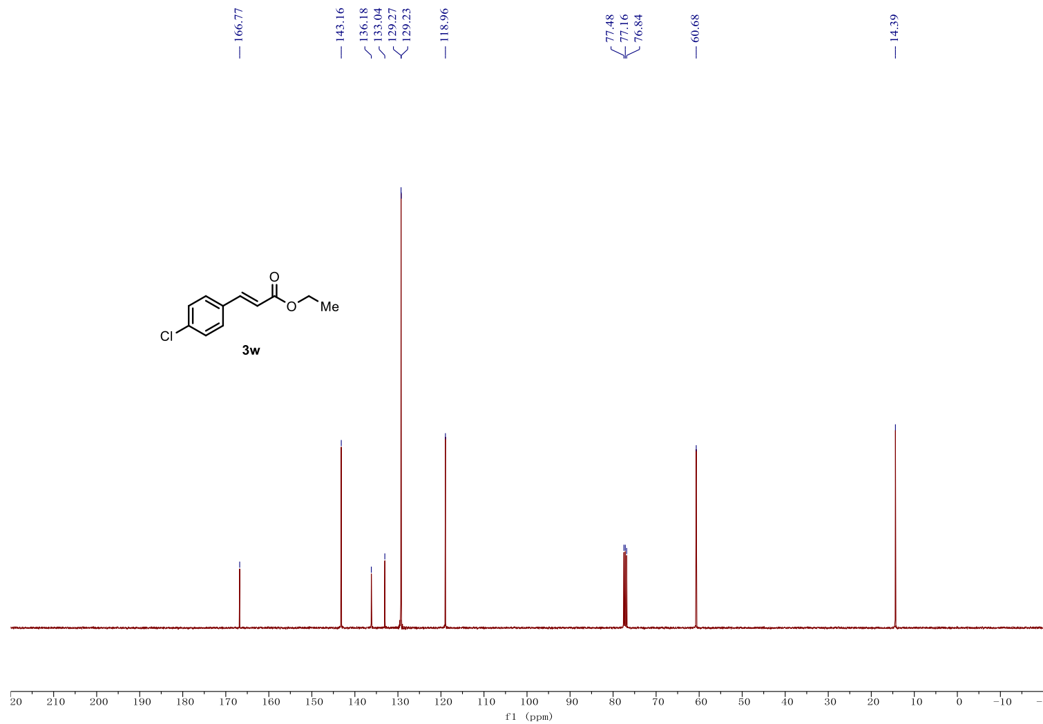
Figure S49. ^{13}\text{C}\{^1\text{H}\} NMR (101 MHz, \text{CDCl}_3 , 298 K) of ethyl ( E )-3-(4-chlorophenyl)prop-2-enoate ( 3w ).
