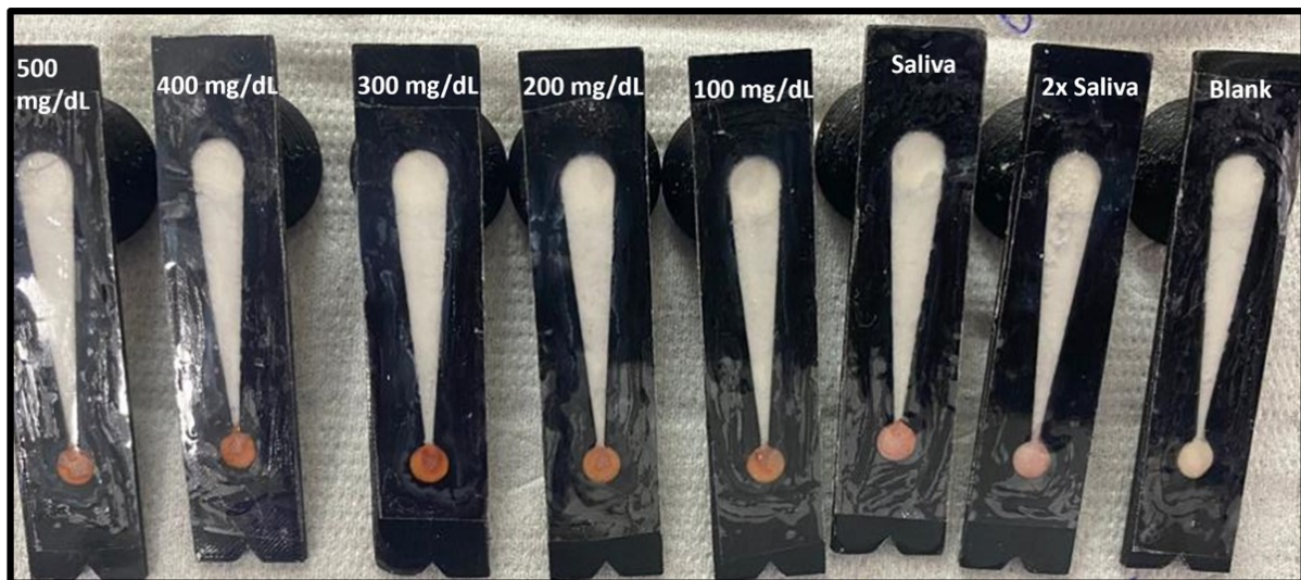
Supplement Fig. S2: Rear view of the strip showing color change with respect to different saliva samples.
