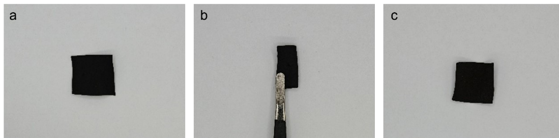
(a), before folding; (b) folding 180 degrees; (c) after folding.
