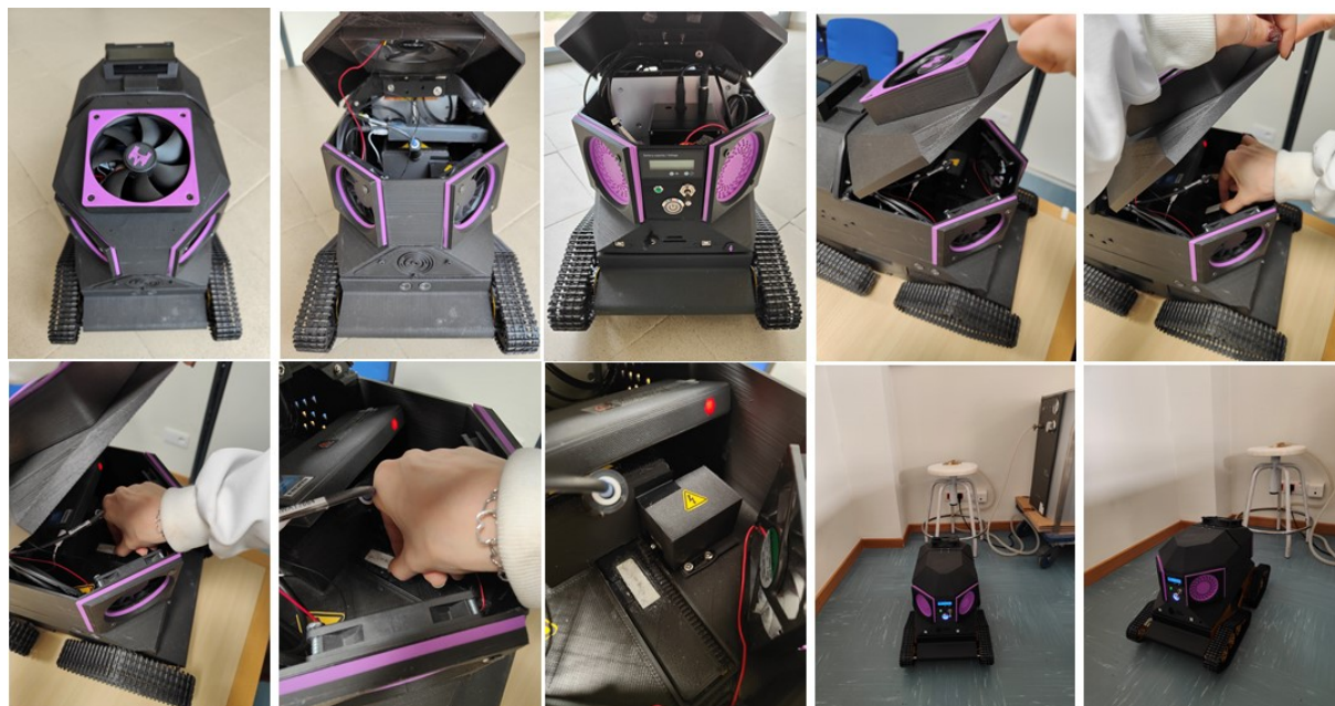
Figure S32. Preparing the mobile platform for the TATP detection experiments.
