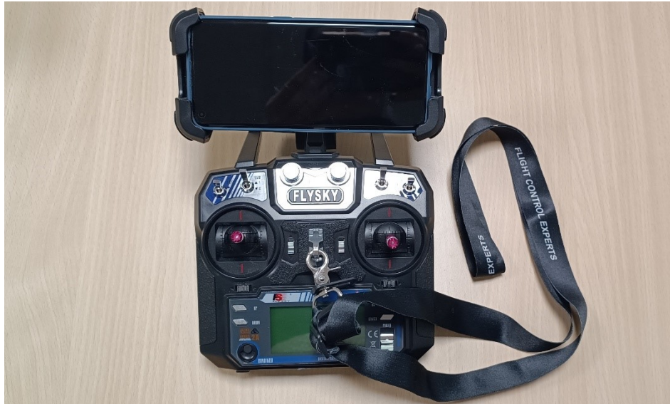
Figure S34. Flysky FS-i6 Radio System Transmitter with mobile device mounting bracket + OPPO Find X3 Pro mobile phone.
