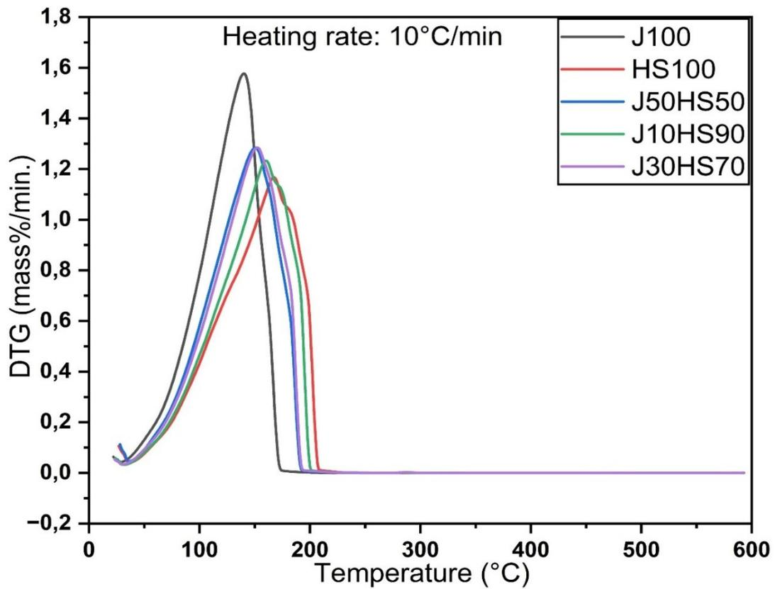
Fig. 3 DTG profiles of tested fuel samples.
