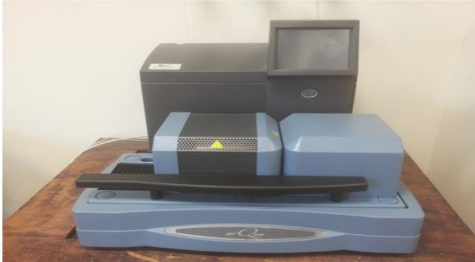
**Fig. 1 (a)** Photographic view of the SDT Q600 TA.
