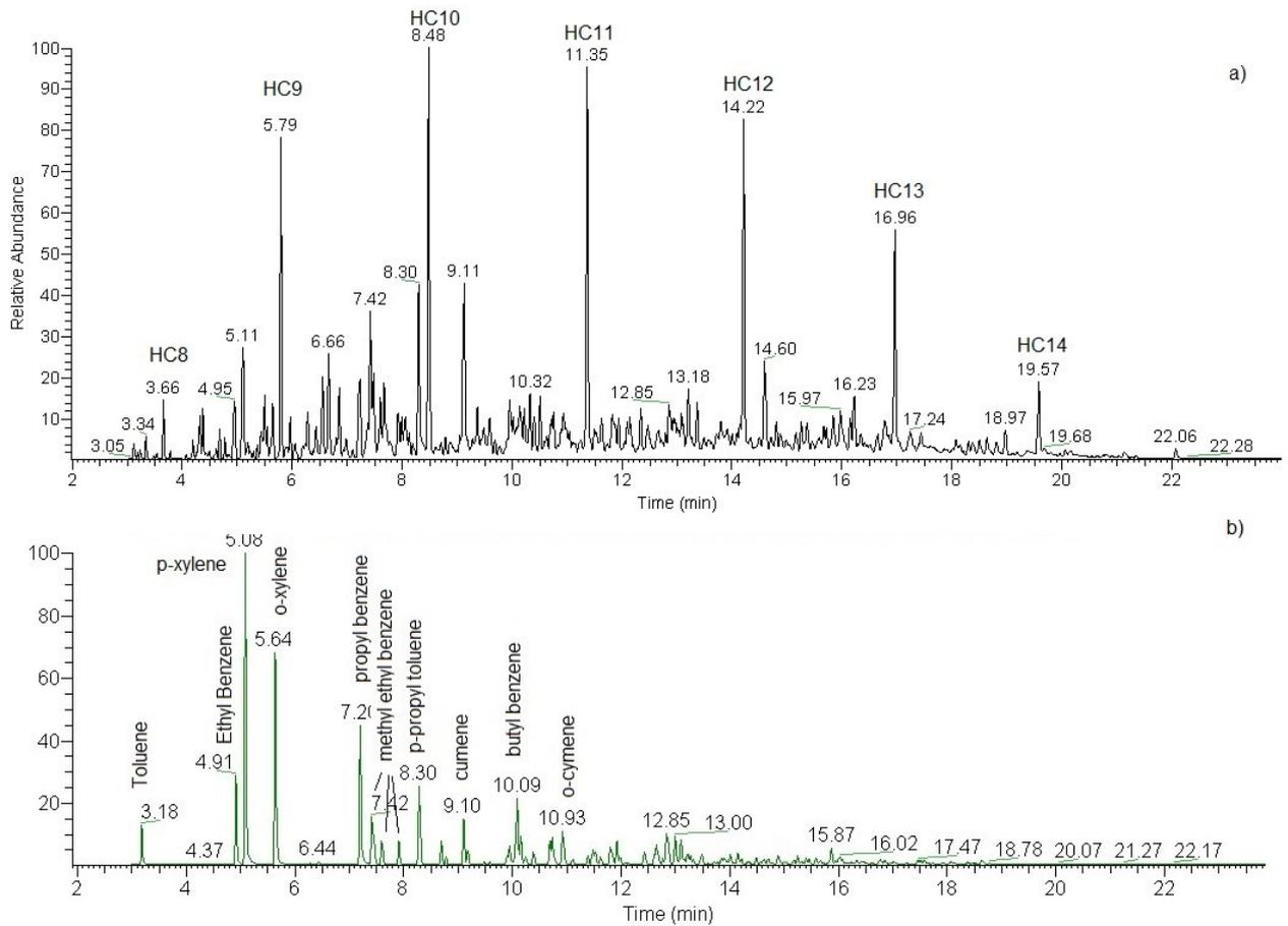
**Figure 7** JET A-1 (J100) Chromatogram (a) TIC, (b) ion extract m/z 91 obtained by GC-MS analysis.
