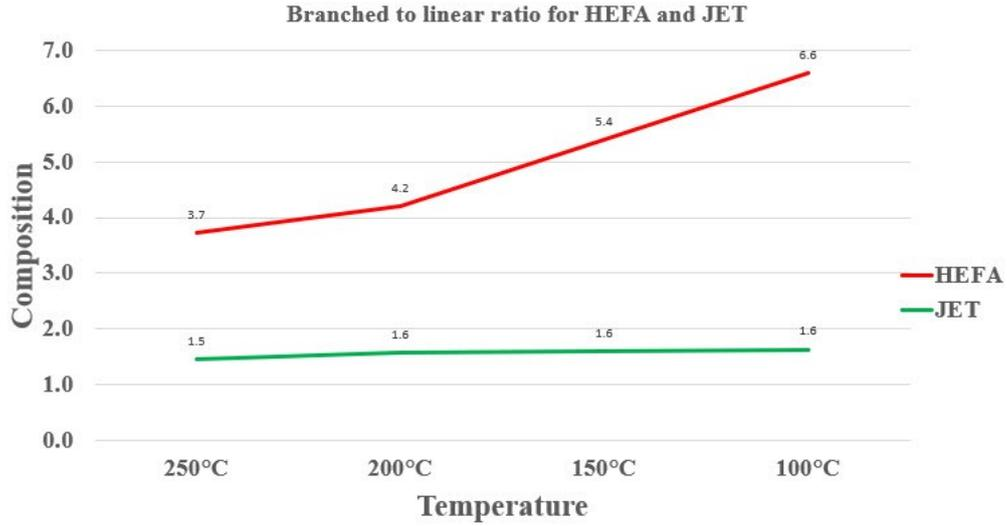
**Fig. 6** Branched to linear hydrocarbons ratio for HEFA and JET as a function of injector temperature.
