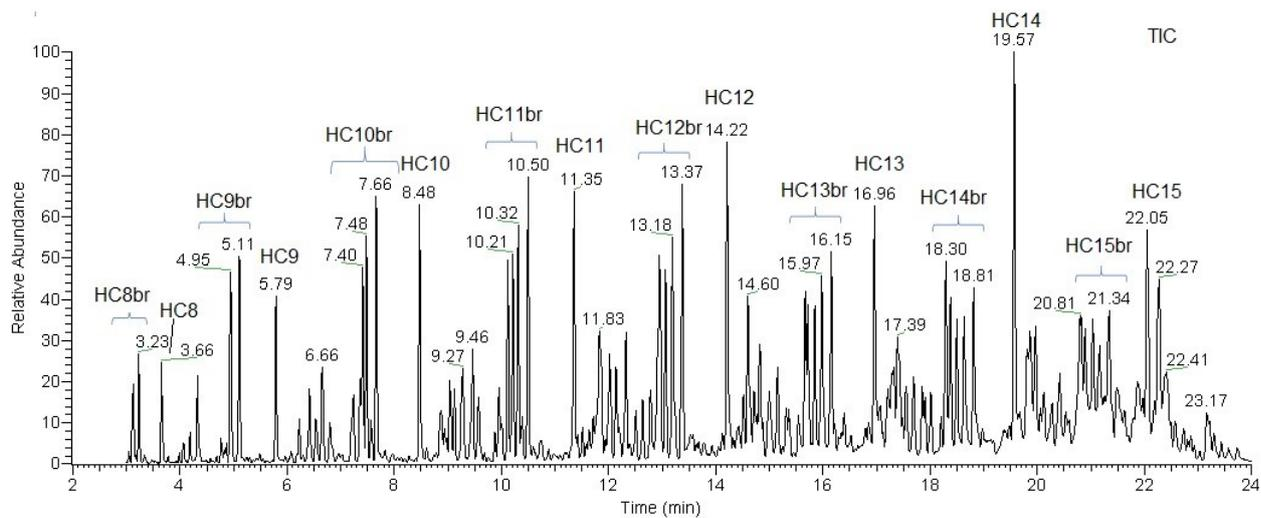
**Figure 8** HEFA-SAF (HS100) Chromatogram (TIC) obtained by GC-MS analysis.
