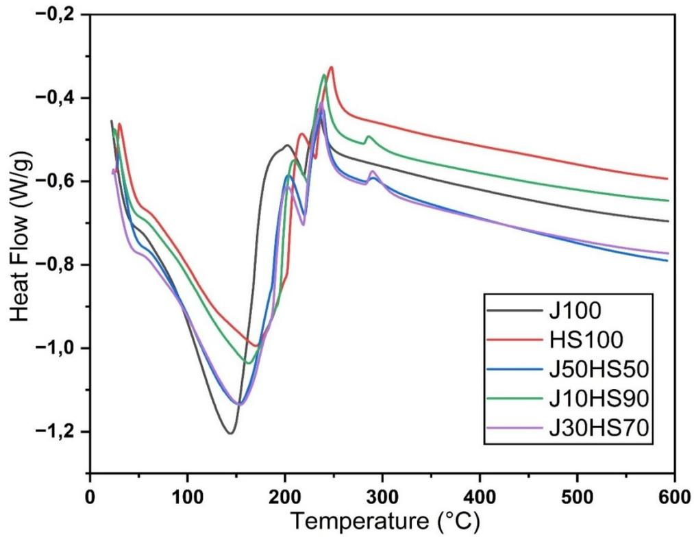
Fig. 4 DSC combustion curves of tested fuel samples.
