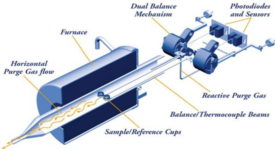
**Fig. 1 (b)** Schematic view of the TGA device used.
