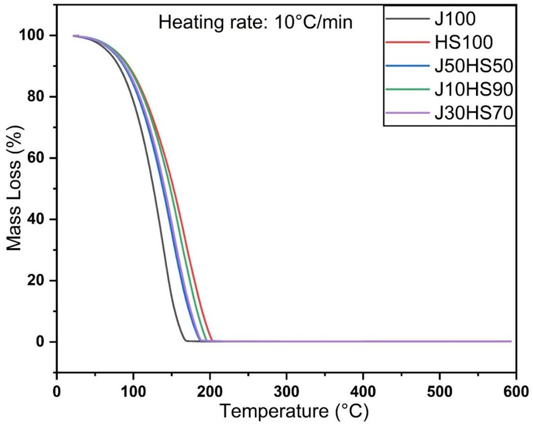
Fig. 2 TGA profiles of tested fuel samples.
