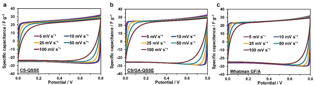
**Fig. S3** CV curves (at sweep rate 5 – 100  $\text{mV s}^{-1}$ ) for EDLCs with (a) CS-QSSE, (b) CS/GA-QSSE, and (c) Whatman GF/A glass fiber separator.
