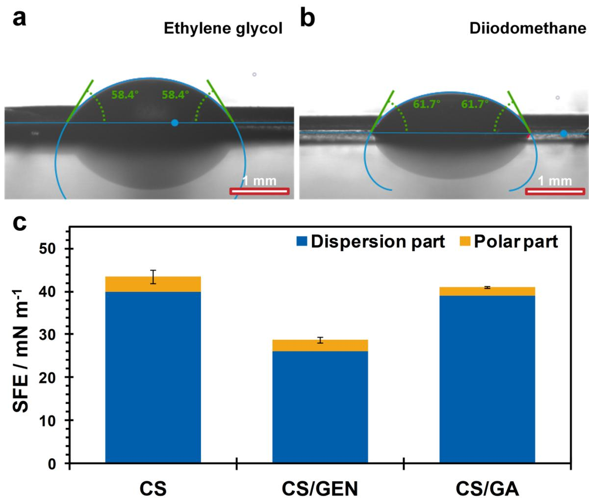
**Fig. S1** Estimated equilibrium contact angles for CS/GEN membrane with (a) ethylene glycol and (b) diiodomethane as a drop liquid. (c) Surface free energy (SFE) of the investigated chitosan-based membranes.
