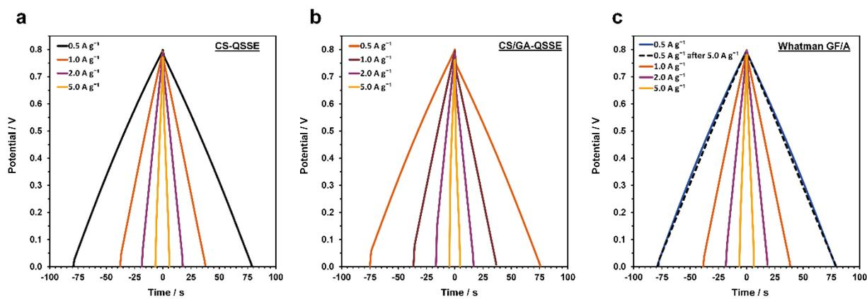
**Fig. S4** Galvanostatic charge/discharge curves at the different current densities for EDLCs with (a) CS-QSSE, (b) CS/GA-QSSE, and (c) Whatman GF/A glass fiber separator.
