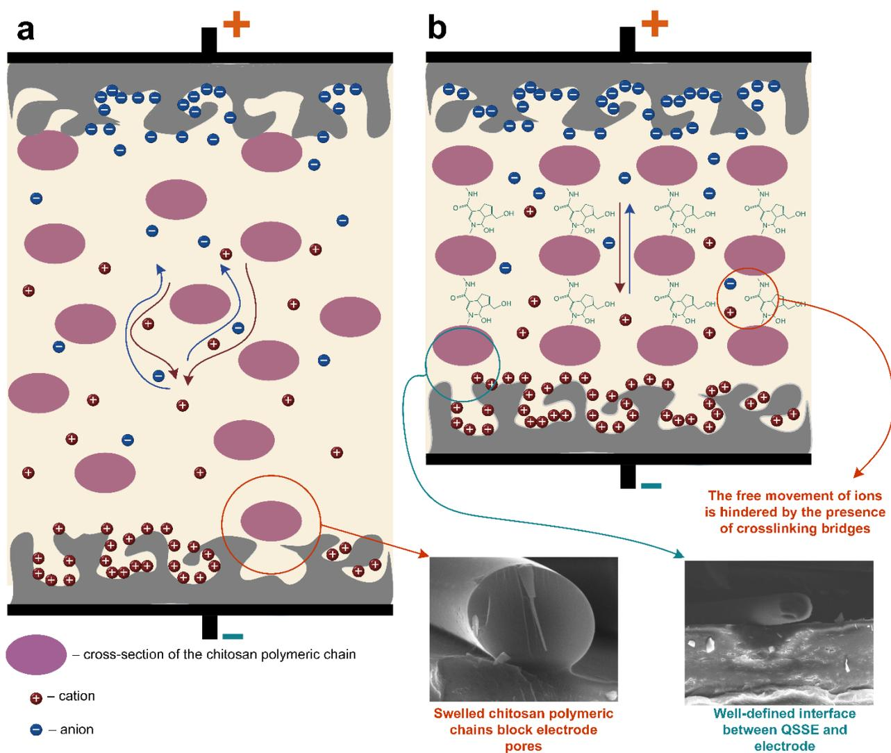
**Fig. S6** Schematic representation of possible differences in charge storage phenomena within operational EDLCs: (a) chitosan-based QSSE without crosslinking and (b) chitosan-based QSSE crosslinked with genipin.
