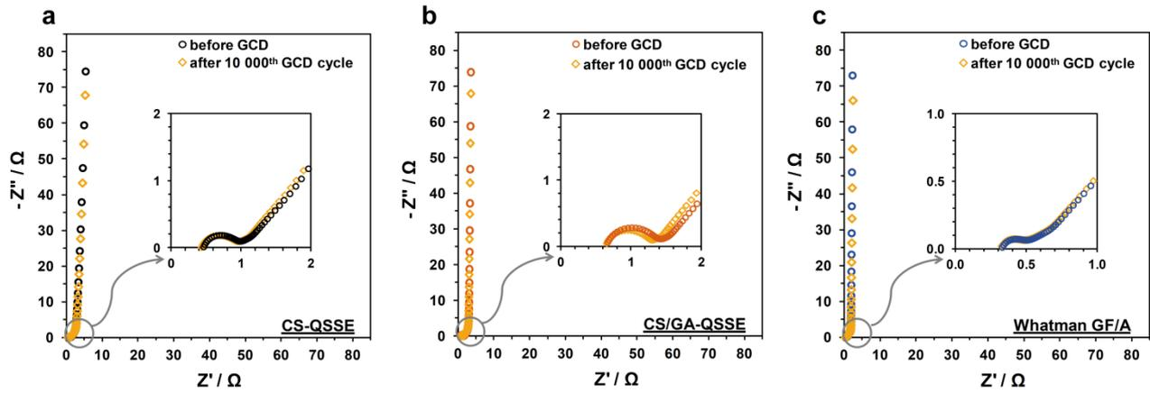
**Fig. S2** AC impedance spectra for capacitors with: (a) CS-QSSE, (b) CS/GA-QSSE, and (c) Whatman GF/A glass fiber separator.
