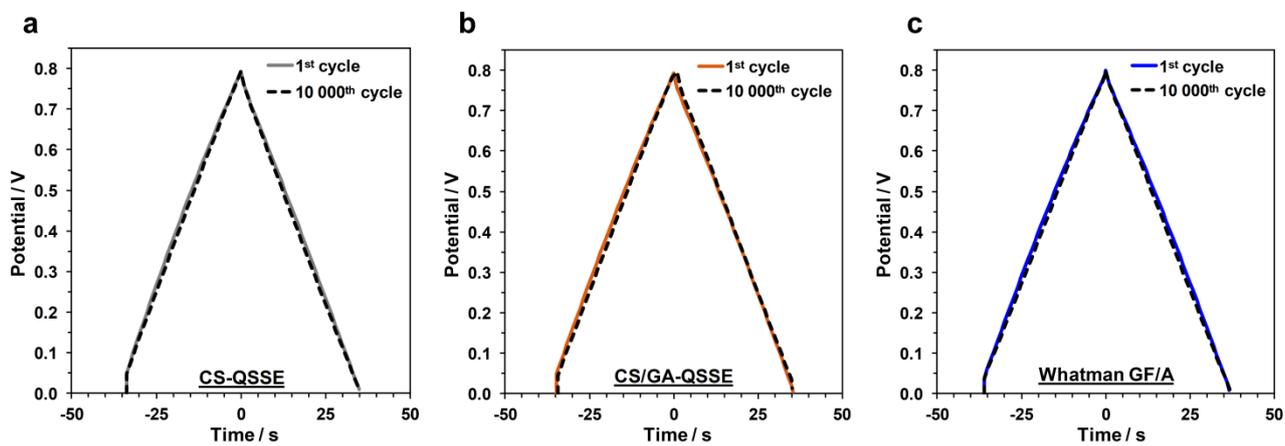
**Fig. S5** Galvanostatic charge/discharge curves at the 1<sup>st</sup> and 10,000<sup>th</sup> cycle (at 1 A g<sup>-1</sup>) for EDLCs with (a) CS-QSSE, (b) CS/GA-QSSE, and (c) Whatman GF/A glass fiber separator.
