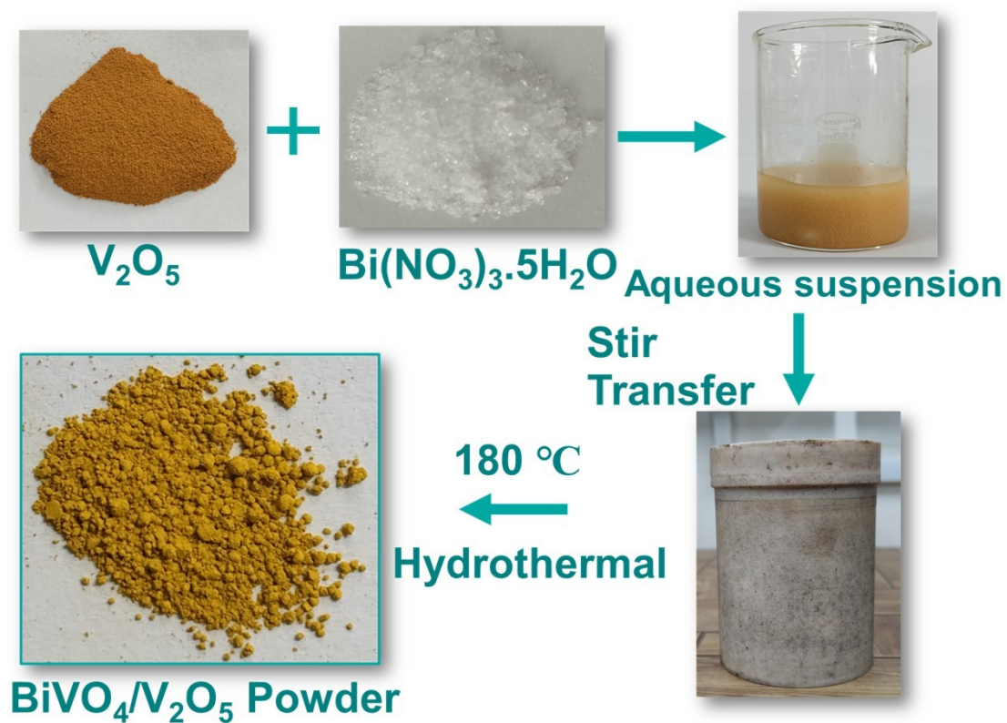
Scheme S1 Synthesis process of the \text{BiVO}_4/\text{V}_2\text{O}_5 heterostructures.
