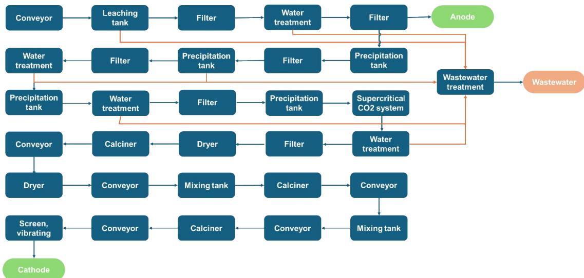
Figure S15 Detailed process and equipment usage for traditional lithium recovery process.
