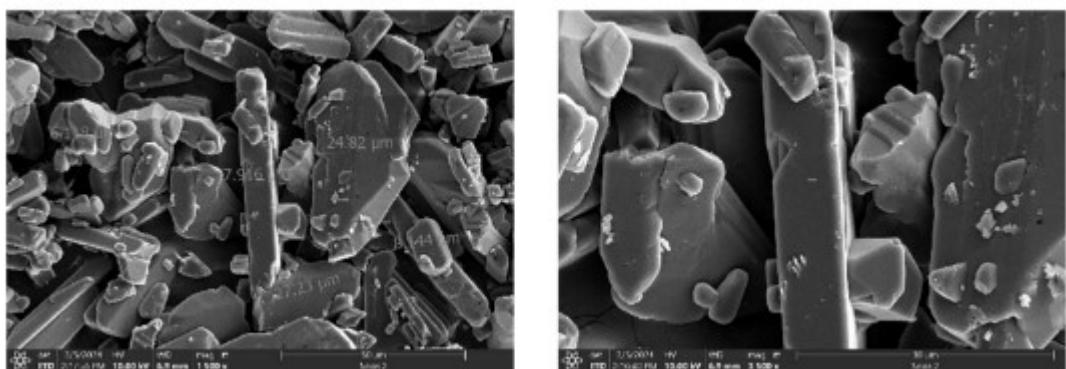
Figure S 8 The morphology for commercial lithium carbonate.
