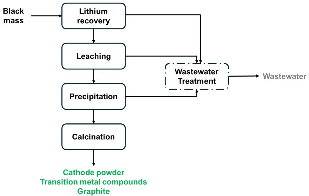
Figure S12 Process diagram of a TPA-lithium recovery process. Solid boxes denote common unit operations; dashed box denotes optional unit operation; green denotes products; grey denotes wastes.
