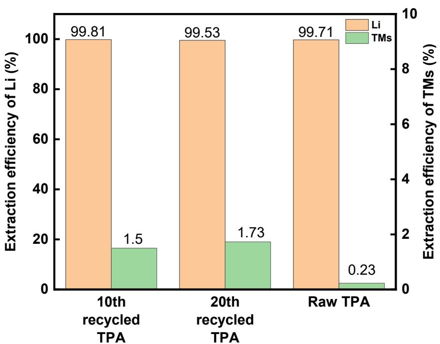
Figure S11 Extraction efficiency comparison for used TPA and raw TPA.
