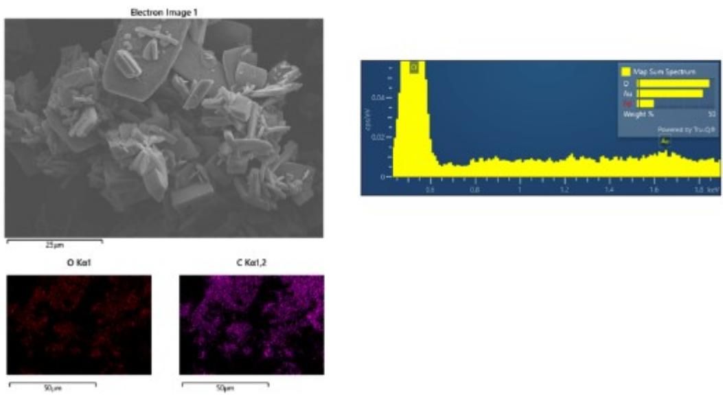
Figure S 7 EDS mapping for Li<sub>2</sub>TP.
