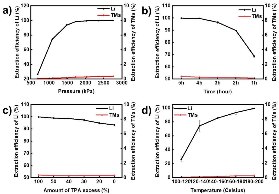
Figure S2 The extraction efficiency for lithium and impurity from NMC622 under a) different pressure, b) different time, c) different amount of TPA excess, and d) different temperature.
