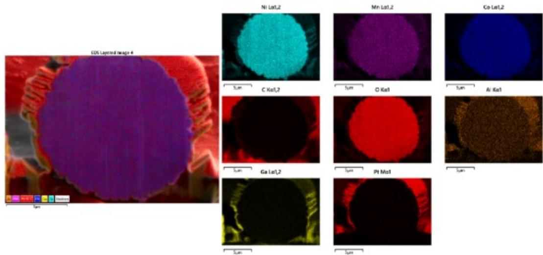
Figure S 5 The EDS mapping for virgin NMC622 cathode powder.
