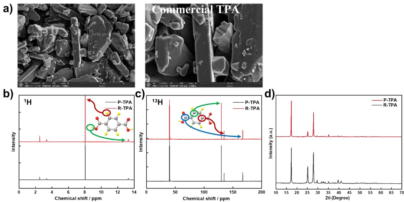
Figure S10 a)SEM images for recovered TPA and commercial TPA, b)  $^1\text{H}$  NMR comparison for pristine (P-TPA) and recycled TPA (R-TPA), c)  $^{13}\text{C}$  NMR comparison for P-TPA and R-TPA, d) XRD comparison for P-TPA and R-TPA.
