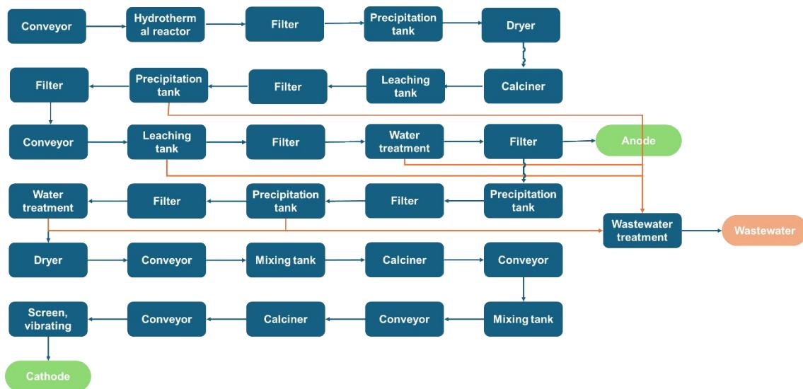
Figure S13 Detailed process and equipment usage for TPA-lithium recovery process.
