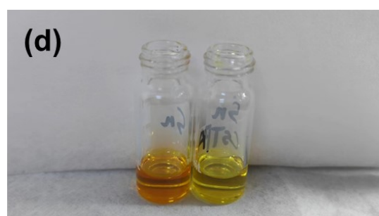
Figure S4. The digital pictures of \text{SnI}_2 solution with (right) and without (left) CsTFA doped placed in ambient condition ( 50-60% RH, 20°C ) for (a) 0min (b) 5min (c) 10min (d) 30min.
