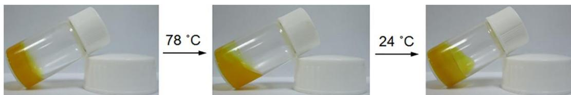
**Fig. S12.** Photographs of the gel-sol phase transition of the hydrogel prepared by PWV<sup>4-</sup> and CPR<sup>2+</sup> upon heating and then cooling.
