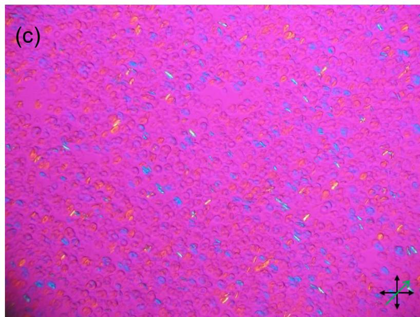
Figure S2 Optical microscopic images of CNC-PEGDA2k particles at wet state with lower magnification (a) BF image, (b) polarized image (c) polarized image with 1<sup>st</sup> order retardation plate ( $\lambda=530$  nm). Direction of polarizer and analyser is shown by arrows.
