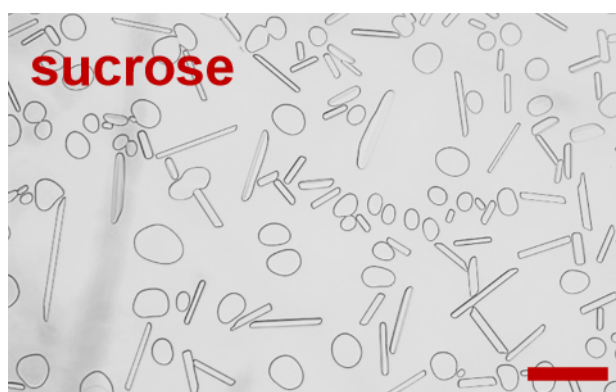
Fig. S9. Sucrose-assisted DIS assay images for 40 wt % sucrose solution. The scale bar is 100 μm.
