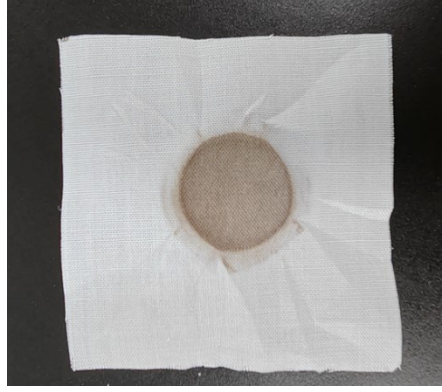
Figure S12. Testing the staining of white standard friction cloth with a color fastness friction tester.
