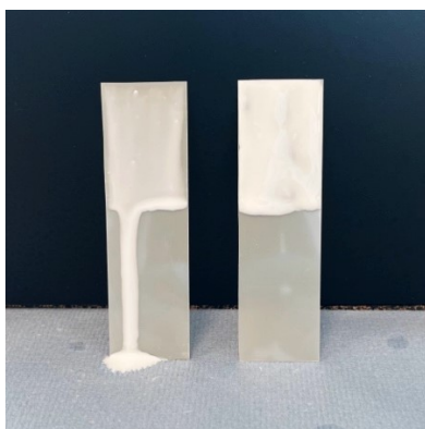
Figure S3. Sagging processes of A0 (left) and A100 (right). A volume of 0.2 mL was used on both cases.
