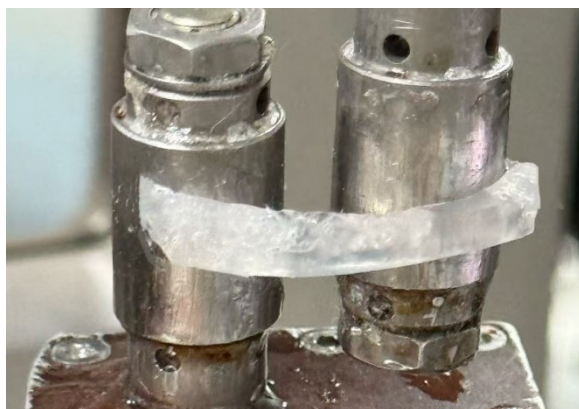
Figure S14: Photograph of the dual-pin grip configuration used for uniaxial extensional testing. Strip specimens were mounted by wrapping each end around a cylindrical post to provide frictional anchoring and to minimize slip. The gauge section was defined as the free span between the two posts.
