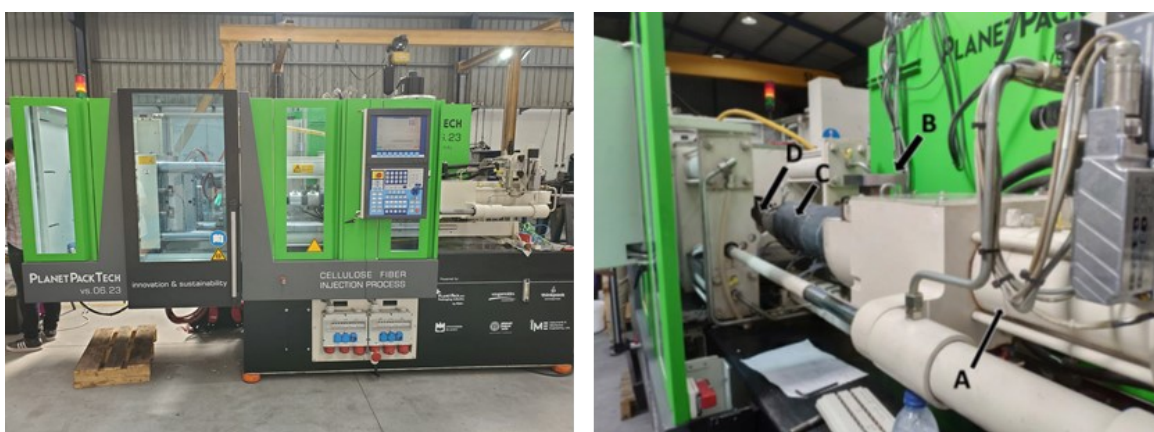
Fig. S1. General view of the Injection Prototype Equipment coupled to a Closing Heating Mould System (left image) and more detailed expansion view (right image) showing the hydraulic system for closing the mould (A), Automated Feeding System (hopper, B), extruder heating elements (C) and the Injection Nozzle (D).
