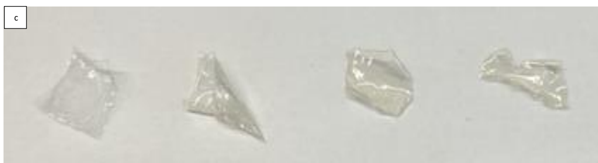
Figure S12: Films F-0, F-3 and F-4 (a) 30 s and (b) 24 h after submerged in 1% NaOH solution. (c) Films F-0, F-1, F-3 and F-4 72 h after submerged in 1% NaOH solution.
