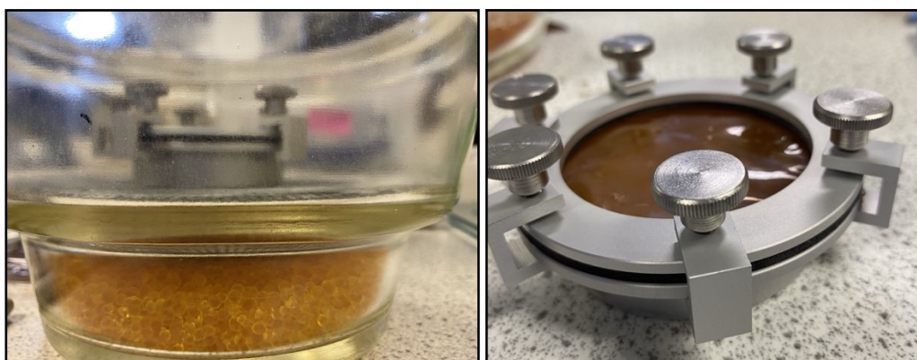
Figure S2. Image of the set-up in the laboratory for water vapour permeability (WVP) experiments using a permeability cup and a glass desiccator with silica beads, maintained at 25.7 \pm 1.1 °C and 37.7 \pm 3.8\% relative humidity, monitored using a digital hygrometer and thermometer.
