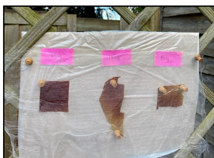
Figure S4. Images of the degradation set-ups (A) the compost bin utilised outside, (B) the set-up for laboratory soil degradation experiments, (C) the soil deposited on a large glass plate to search for degradation products, (D) outside UV degradation set-up, (E) the inside of the compost bin, with samples attached to twine and (F) the seawater degradation experiment in the laboratory.
