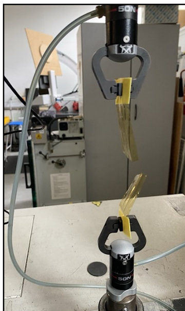
Figure S6. Image of tensile strength experiments, with masking tape used on the ends of the sample to prevent cracking and slippage.
