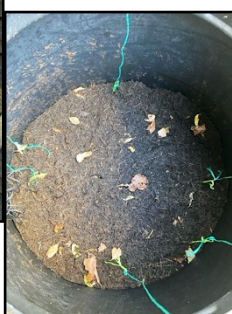
Figure S4. Images of the degradation set-ups (A) the compost bin utilised outside, (B) the set-up for laboratory soil degradation experiments, (C) the soil deposited on a large glass plate to search for degradation products, (D) outside UV degradation set-up, (E) the inside of the compost bin, with samples attached to twine and (F) the seawater degradation experiment in the laboratory.
