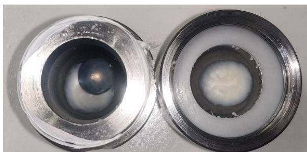
Figure S7. View of the milling jar after the mechanochemical hydrolysis reaction using 1 equiv. of NaCl as an additive under otherwise optimised reaction conditions (vide supra).
