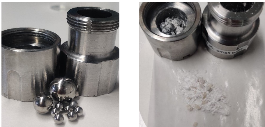
Figure S8. Views of the milling jar after the mechanochemical hydrolysis reaction using smaller balls, under otherwise optimised reaction conditions (vide supra).
