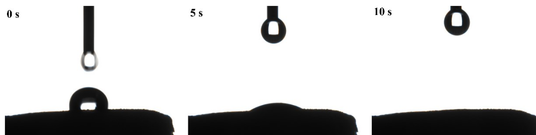
Fig. S7 Water contact angle tests of CWRR
