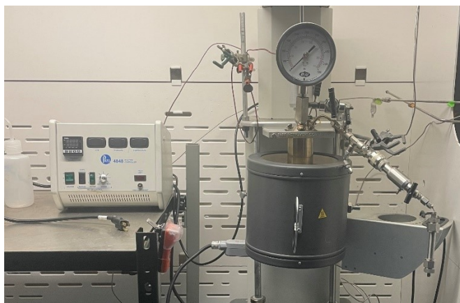
Figure S10. Parr reactor vessel used for SCWO experiments
