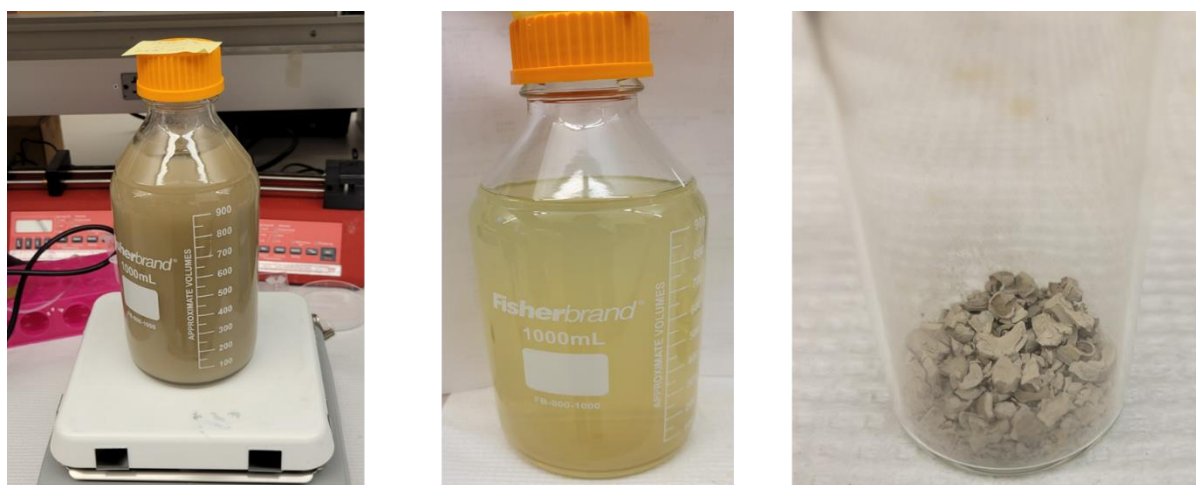
Figure S2. Bulk olivine dissolution experiment of 15 g of olivine in 1 liter of BPMED acid (left). BPMED solution after 2 weeks of dissolution after solid removal (middle). Solid residue collected after exposure to BPMED acid for 2 weeks (right)
