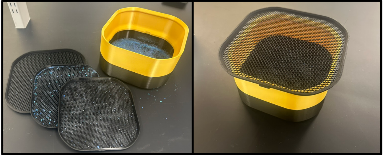
Figure S3. 3D printed particle sieve to homogenise the shredded material before drying and extrusion. The design files associated to the sieves can be found here: https://makerworld.com/en/models/661908-modular-sieve-mesh#profileId-589154 .
