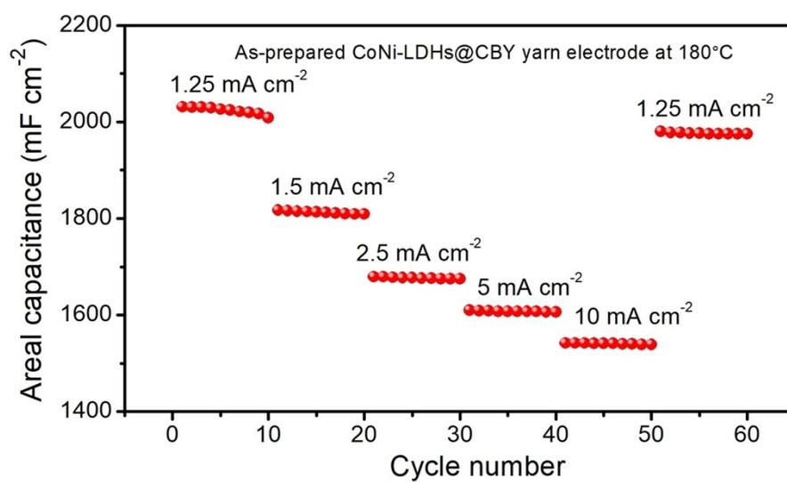
**Fig. S6.** Rate performance of the as-prepared CoNi-LDHs@CBY yarn electrode at 180°C.
