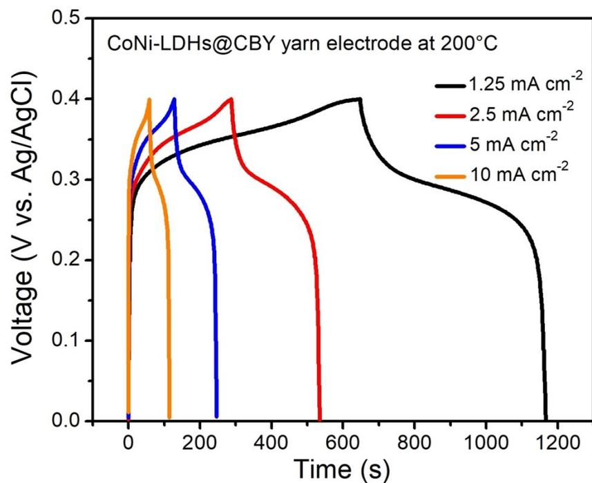
**Fig. S5.** GCD profiles of CoNi-LDHs@CBY yarn electrode at 200°C.
