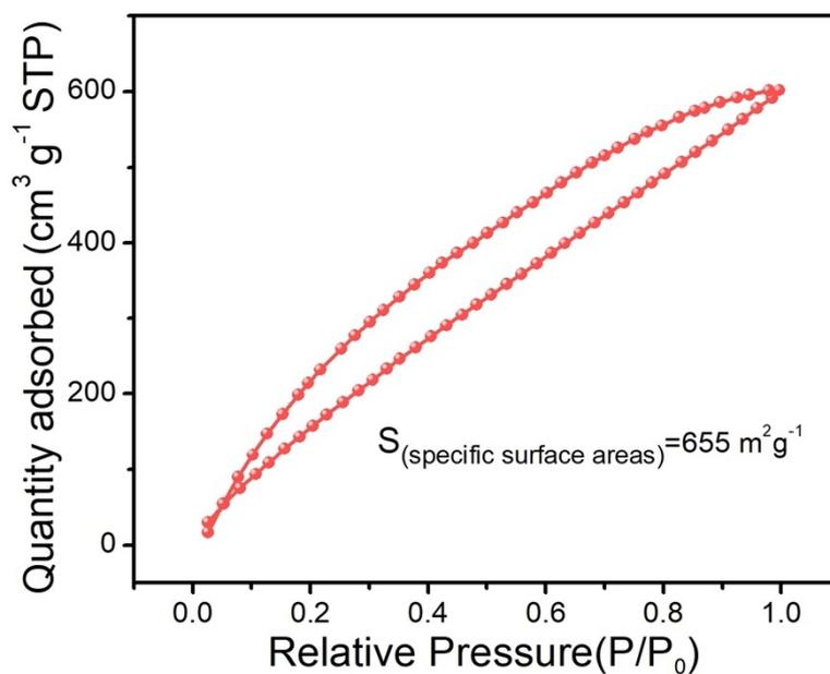
**Fig. S1.** N<sub>2</sub> adsorption-desorption curves and specific surface areas of CoNi-LDHs@CBY yarn electrode.
