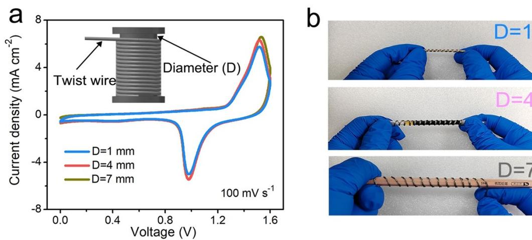
**Fig. S12.** (a) CV curves and (b) photograph of the flexible CoNi-LDHs@CBY//S-CNPs@CBY device under different twist twine diameters.
