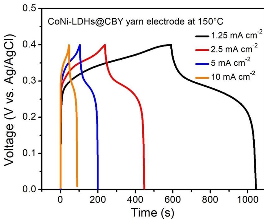
**Fig. S4.** GCD profiles of CoNi-LDHs@CBY yarn electrode at 150°C.
