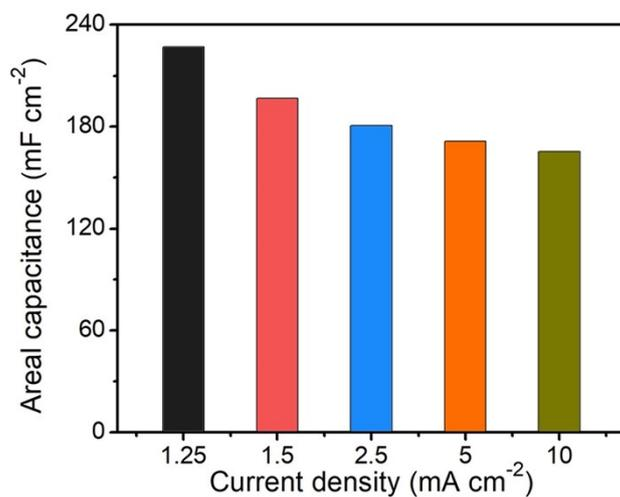
**Fig. S10.** The areal capacitance of the flexible CoNi-LDHs@CBY//S-CNPs@CBY device.
