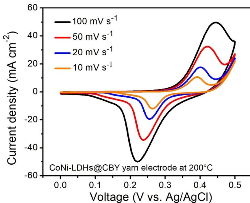
**Fig. S3.** CV curves of CoNi-LDHs@CBY yarn electrode at 200°C.
