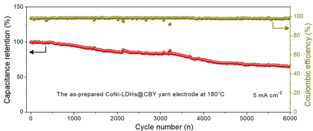
**Fig. S7.** Cycling performance of the as-prepared CoNi-LDHs@CBY yarn electrode at 180°C.
