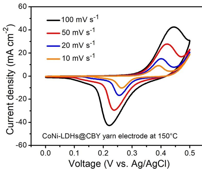
**Fig. S2.** CV curves of CoNi-LDHs@CBY yarn electrode at 150°C.
