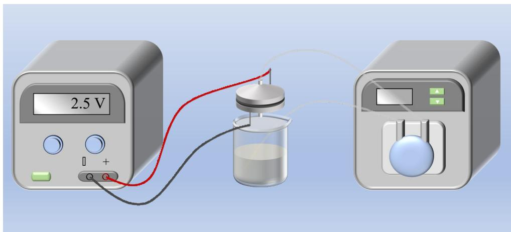
Figure S1 Schematic diagram of an electro-Fenton reaction device
