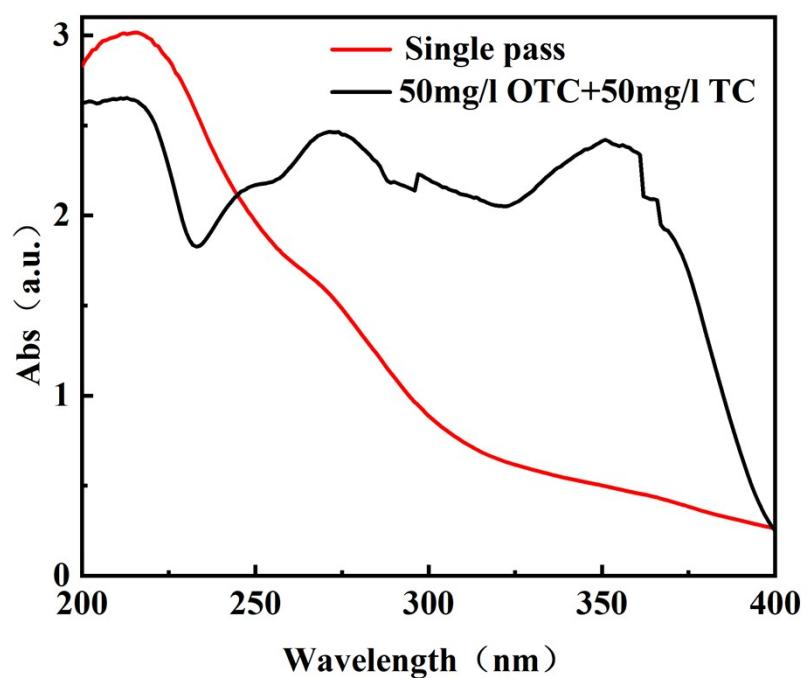
Figure S4 UV-Vis spectra before and after a single passage of 50 mg/l OTC+TC mixed solution through FeS<sub>2</sub>/ACFs membrane
