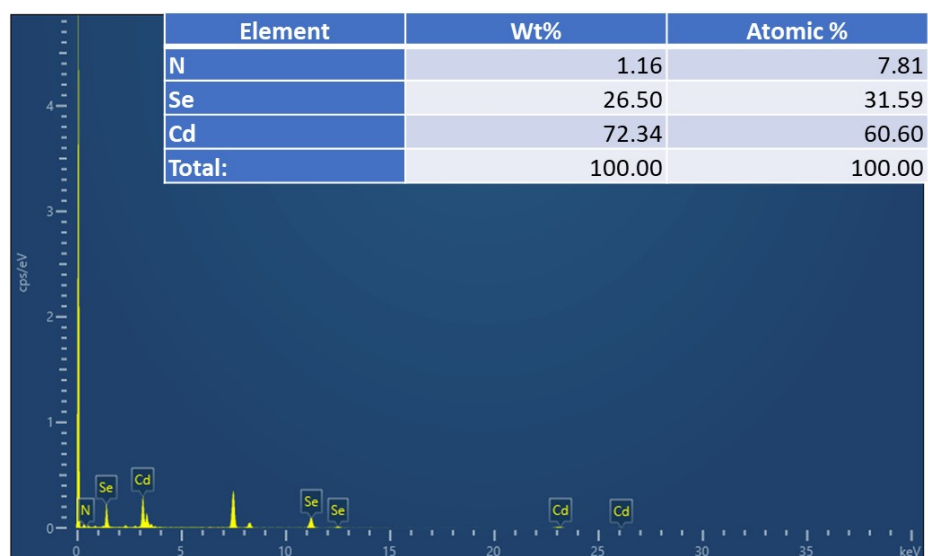
Fig. S6 EDS elemental spectrum and quantification results for selective porous CdSeNS of CdSeNS/CdSNR-6h photoanode.
