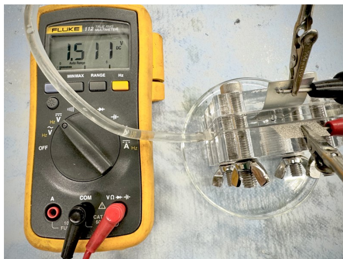
Fig. S19 Photographic image of the voltage meter showing the OCV of ZABs.
