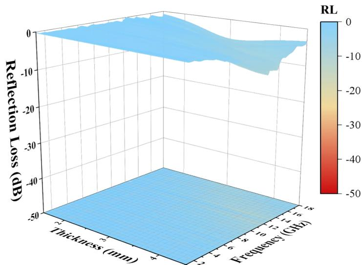
**Figure S8.** Three-dimensional representation and contour RL values versus frequency at different thicknesses samples for grabular PPY-Fe with filler ratio of 10%. Given the close similarities in component between the two samples, the higher performance of PPY-Fe2 compared to reference grabular PPY-Fe (at the same filler loading) was reasonably ascribed to the unique 1D/2D nanostructure of PPY-Fe2 aerogel.
