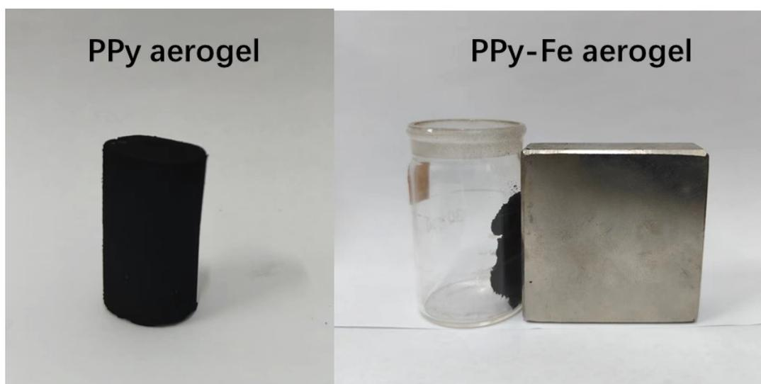
**Figure S2.** Photos of as-prepared pure PPy aerogel (left) and PPy-Fe<sub>2</sub> aerogel. The PPy-Fe<sub>2</sub> sample can be attracted to the external permanent magnet.
