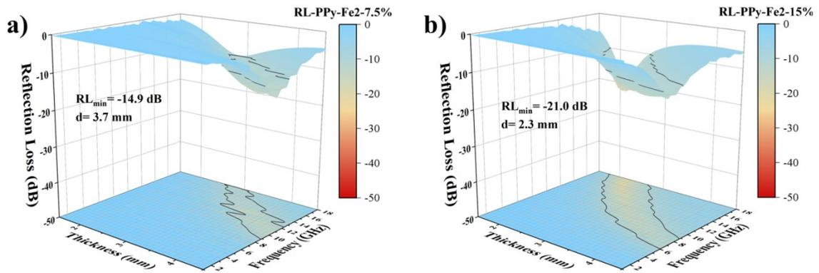
**Figure S7.** Three-dimensional representations and contour RL values versus frequency at different thicknesses samples for PPy-Fe2 with filler ratio of 7.5% and 15%, respectively.
