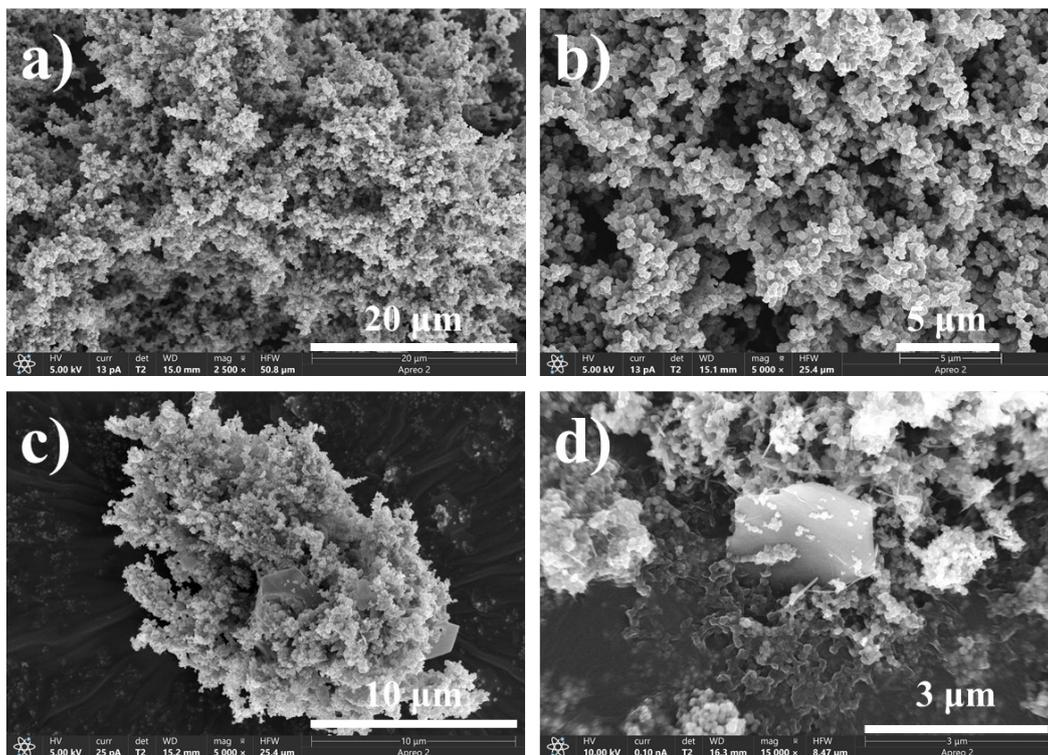
**Figure S1.** Scanning electron microscopy image of pure grabular PPy aerogel (a,b) and grabular PPy-Fe aerogel (c,d). The reference grabular PPy aerogels were prepared by the oxidation of pyrrole with iron(III) chloride in the absence of methyl orange.
