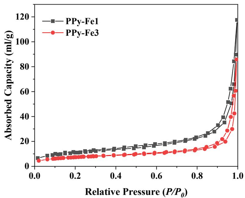
**Figure S3.**  $N_2$  adsorption-desorption isotherms of PPy-Fe1 and PPy-Fe3 samples.
