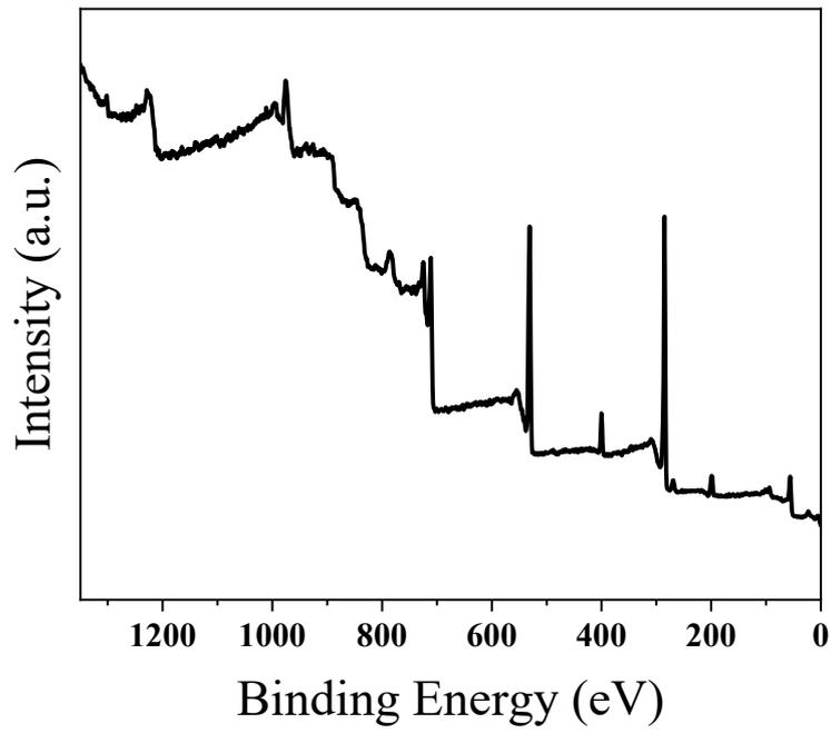
**Figure S5.** Survey XPS spectra of the PPy-Fe sample.
