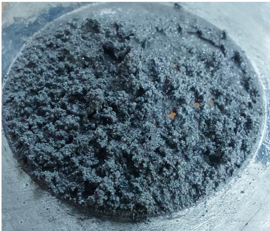
Figure S20. Photograph of zinc anode after long charging the CoILPh 700 zinc-air battery at 5 mA/cm 2 for 72 h
