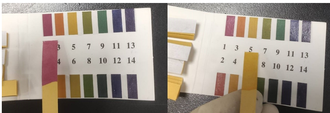
Figure S1: a) 2M AMPS solution pH; b) AMPS-Zn solution pH after adding ZnO
