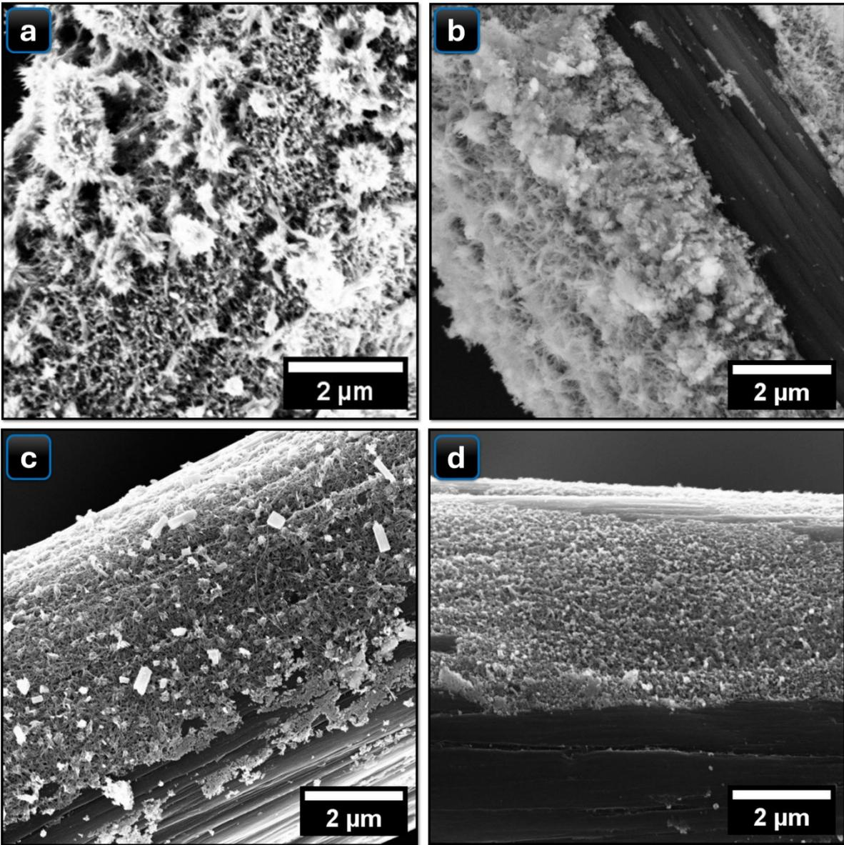
**Figure S3:** The SEM images for a) W@CF, b) W<sub>2</sub>-Bi@CF, c) W-Bi@CF, and d) W-Bi<sub>2</sub>@CF electrodes at low magnification.
