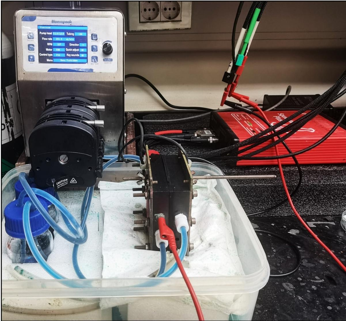
**Figure S2:** A photograph of the assembled VRFB system used in the device measurements.
