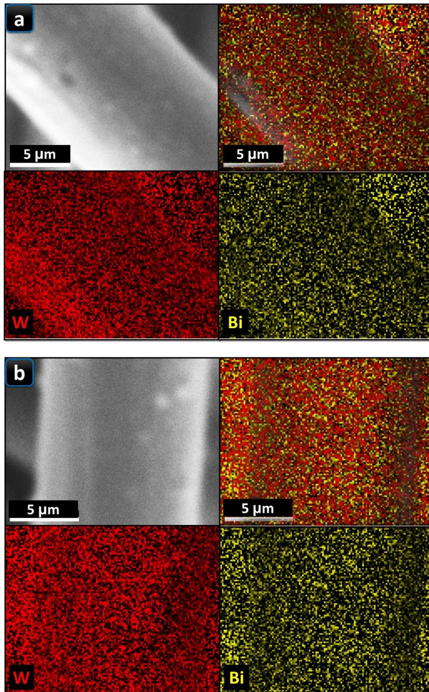
**Figure S4:** The EDS mapping analysis for the W-Bi<sub>2</sub>@CF electrode a) before and b) after the electrochemical CV cycling.
