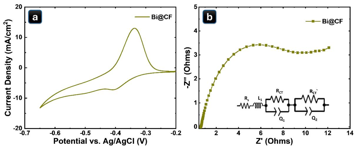
**Figure S8:** a) CV curve at the scan rate of 5 mV/s and b) EIS pattern for Bi@CF electrode in 0.1 M  $V^{2+}$  in 1 M  $H_2SO_4$  solution.
