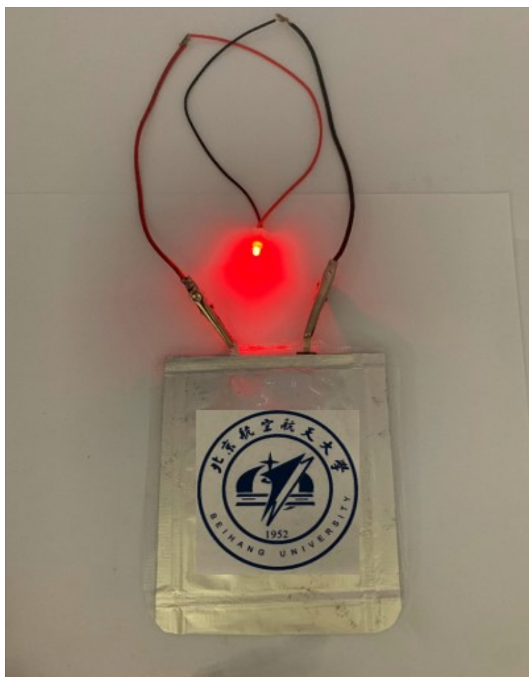
Fig. S17 Photograph of Li/PCL-DDCA-PC electrolyte/LiFePO 4 pouch-type cell lighting up the red LED panel.
