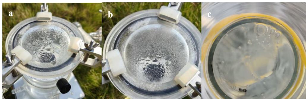
Figure S13. (a) the photo of the top cover of the outdoor experimental setup, (b) vapor condensed in the top cover, and (c) \text{H}_2 bubbles in the volumetric cylinder.
