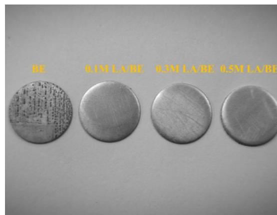
**Fig. S14.** Digital photos of zinc sheets soaked in different concentrations of electrolyte
