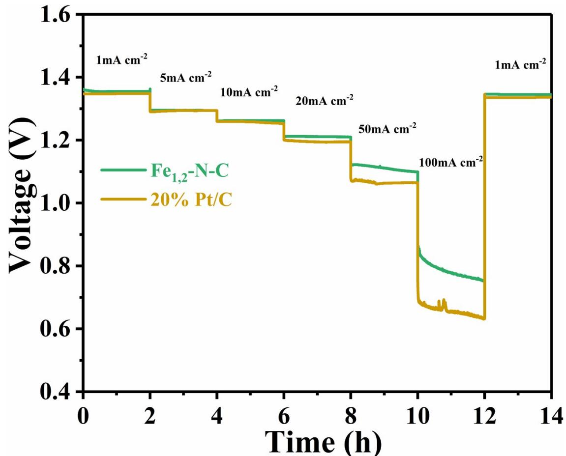
8 **Figure S19.** The galvanostatic discharge curves of the aqueous
