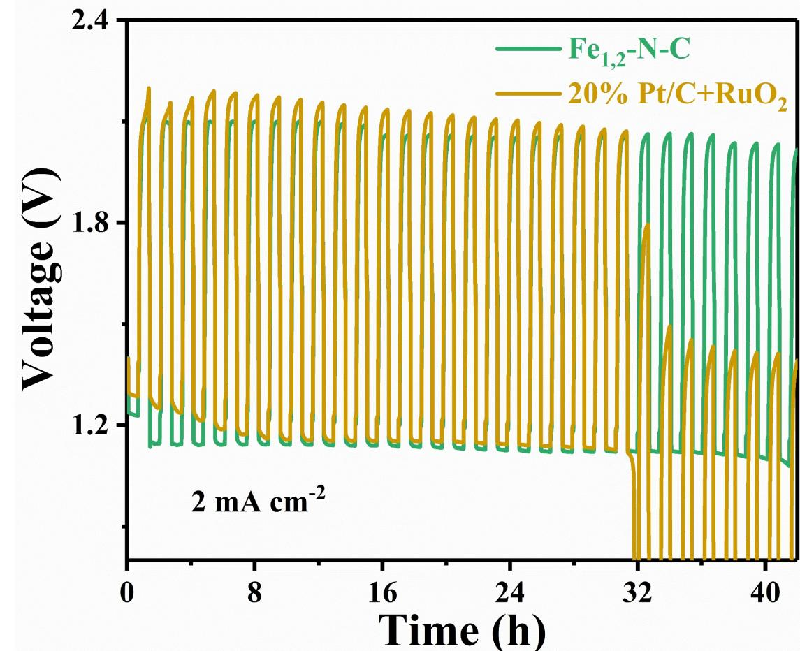
9 **Figure S20.** Charge and discharge curve with  $\text{Fe}_{1,2}\text{-N-C}$  and 20%
