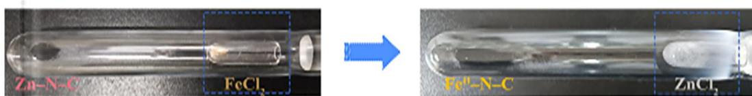
**Figure S1.** Schematic diagram of the experimental preparation of Fe<sup>II</sup>-N-C catalyst.
