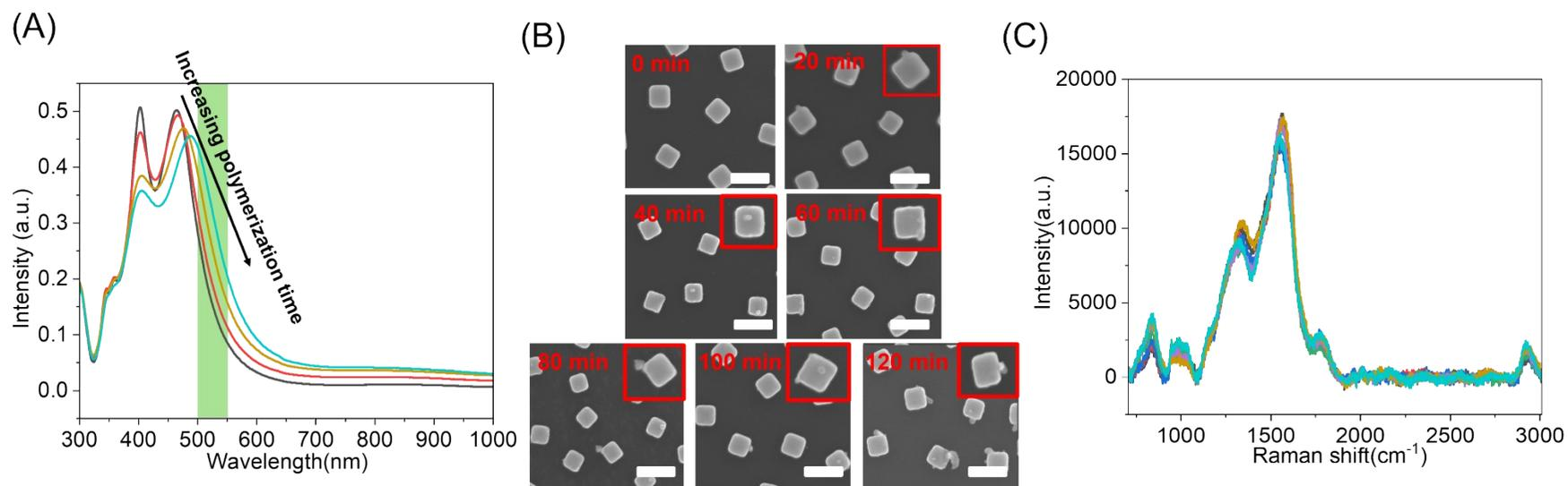
**Figure S17 Lactic acid polymerization of AgNC surface under  $520 \pm 20$  nm wavelength irradiation at  $-12$  °C.** (A) changes in the extinction spectrum of AgNC during polymerization process. (B) characterization of the morphology changes of AgNC during the polymerization process through SEM images. (C) changes in Raman spectra during the polymerization process were used to characterize the amount of polylactic acid formed on AgNC surface. The scale bar was 200 nm.
