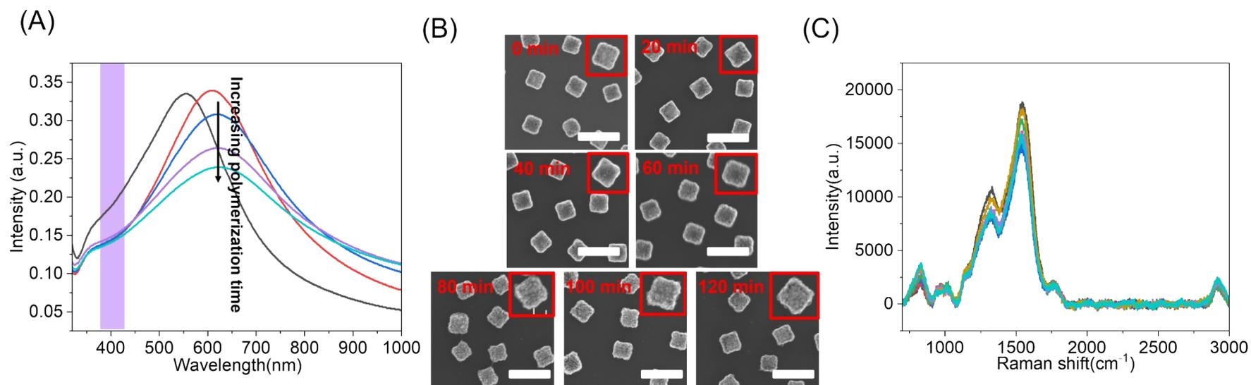
**Figure S21 Lactic acid polymerization of cage-like Au-AgNC surface under  $420 \pm 20$  nm wavelength irradiation at  $-12$  °C.** (A) changes in the extinction spectrum of AgNC during polymerization process. (B) characterization of the morphology changes of AgNC during the polymerization process through SEM images. (C) changes in Raman spectra during the polymerization process were used to characterize the amount of polylactic acid formed on AgNC surface. The scale bar was 200 nm.
