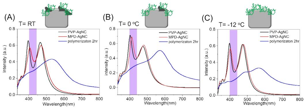
**Figure S5 Changes in optical properties of AgNC during lactic acid polymerization at different temperatures under irradiation. (A) at room temperature. (B) at 0 °C. (C) at -12 °C. Black curve: PVP coated AgNC. Red curve: MPD coated AgNC. Blue curve: AgNC after 2 hours of polymerization.**
