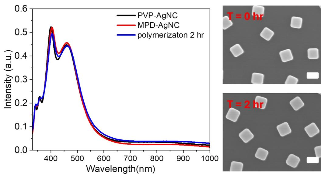
**Figure S6 Changes in optical properties of AgNC during lactic acid polymerization at -12 °C.** And the light source was irradiated on the reaction solution but not on the substrate with AgNC. Black curve: PVP coated AgNC. Red curve: MPD coated AgNC. Blue curve: AgNC after 2 hours of polymerization. And SEM images before and after 2 hours of polymerization showed that there was no lactic acid polymerization and Ag oxidation on the AgNC surface. The scale bar was 100 nm.
