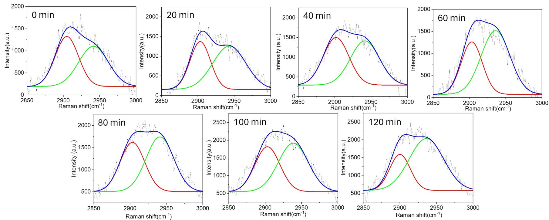
**Figure S22** The multi-curve fitting results of Raman scattering spectra during lactic acid polymerization on cage-like Au-AgNC surface under  $420 \pm 20$  nm wavelength irradiation at  $-12$  °C. The results showed the multi-curve fitting at different polymerization times.
