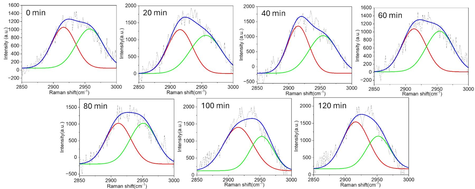
**Figure S20** The multi-curve fitting results of Raman scattering spectra during lactic acid polymerization on AgNC surface under  $600 \pm 20$  nm wavelength irradiation at  $-12$  °C. The results showed the multi-curve fitting at different polymerization times.
