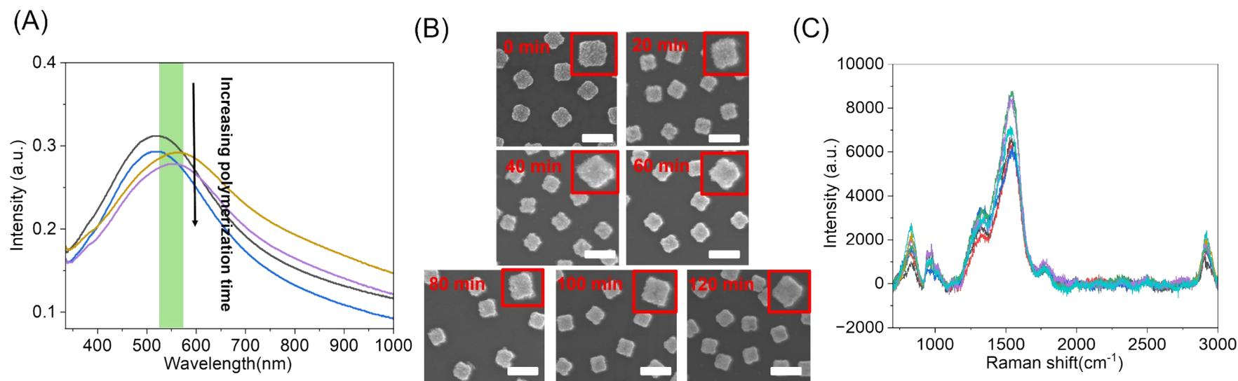
**Figure S29 Lactic acid polymerization of flower-like Au-AgNC surface under  $520 \pm 20$  nm wavelength irradiation at  $-12$  °C.** (A) changes in the extinction spectrum of AgNC during polymerization process. (B) characterization of the morphology changes of AgNC during the polymerization process through SEM images. (C) changes in Raman spectra during the polymerization process were used to characterize the amount of polylactic acid formed on AgNC surface. The scale bar was 200 nm.
