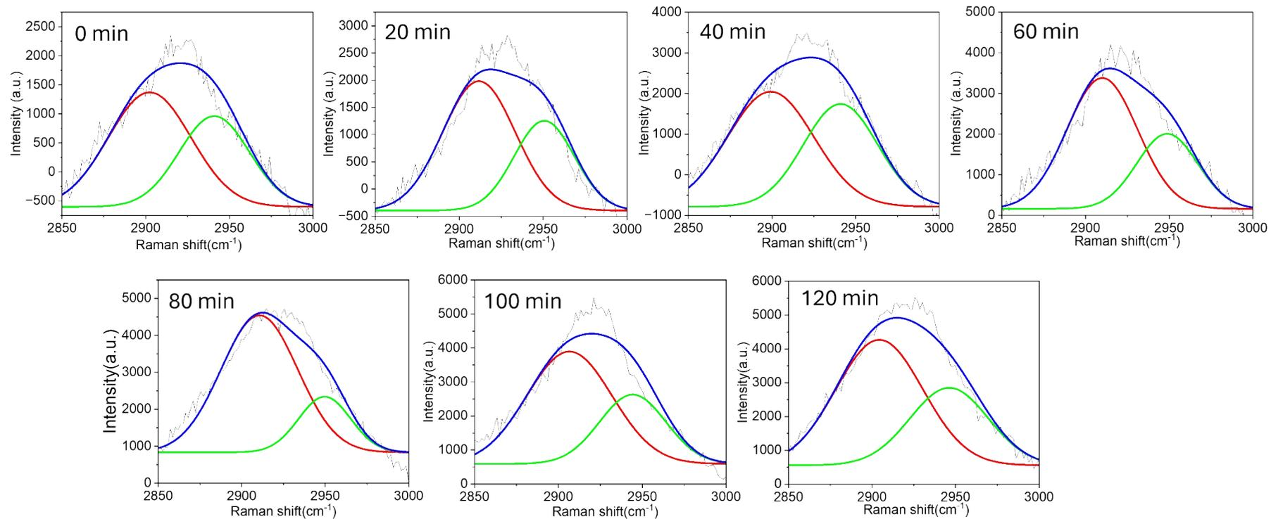
**Figure S12** The multi-curve fitting results of Raman scattering spectra during lactic acid polymerization on AgNC surface under  $420 \pm 20$  nm wavelength irradiation at  $-12$  °C. The results showed the multi-curve fitting at different polymerization times.
