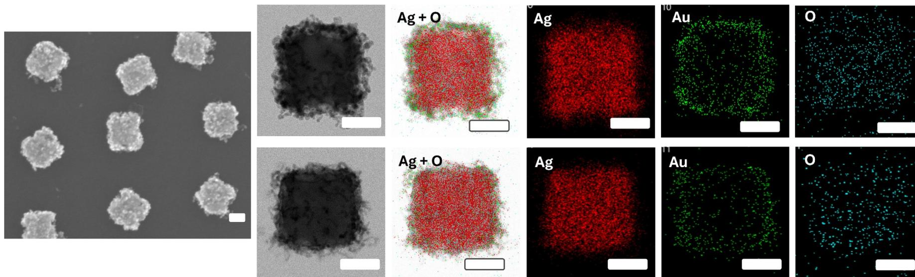
**Figure S16** Characterization of lactic acid polymerization on flower like Au-AgNC surface under -12 °C under irradiation by SEM, TEM, and EDX analysis. The results showed that Ag oxidation on flower-like Au-AgNC surface can be completely inhibited. The scale bar was 50 nm.
