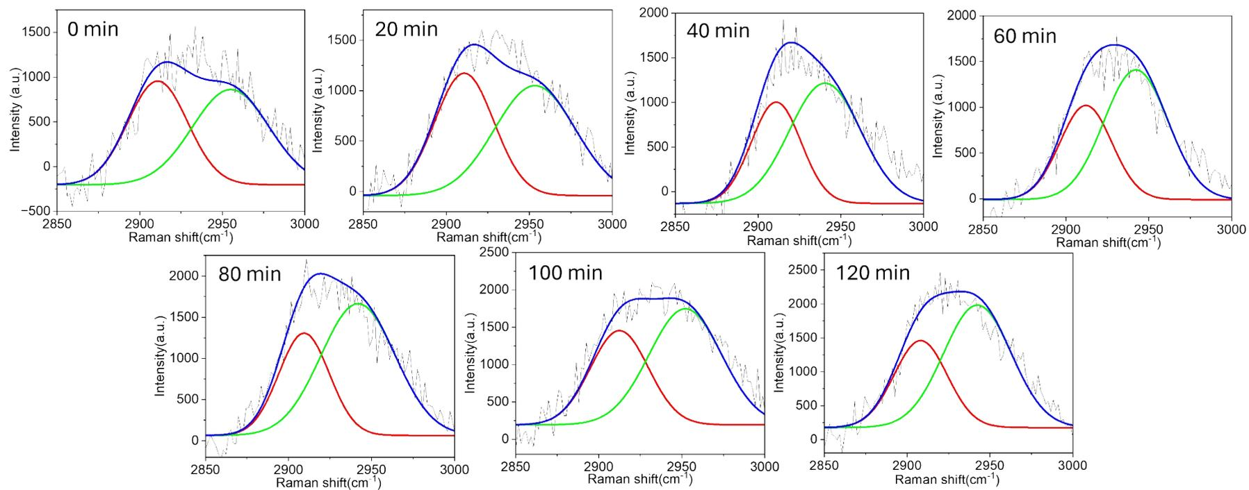
**Figure S18** The multi-curve fitting results of Raman scattering spectra during lactic acid polymerization on AgNC surface under  $520 \pm 20$  nm wavelength irradiation at  $-12$  °C. The results showed the multi-curve fitting at different polymerization times.
