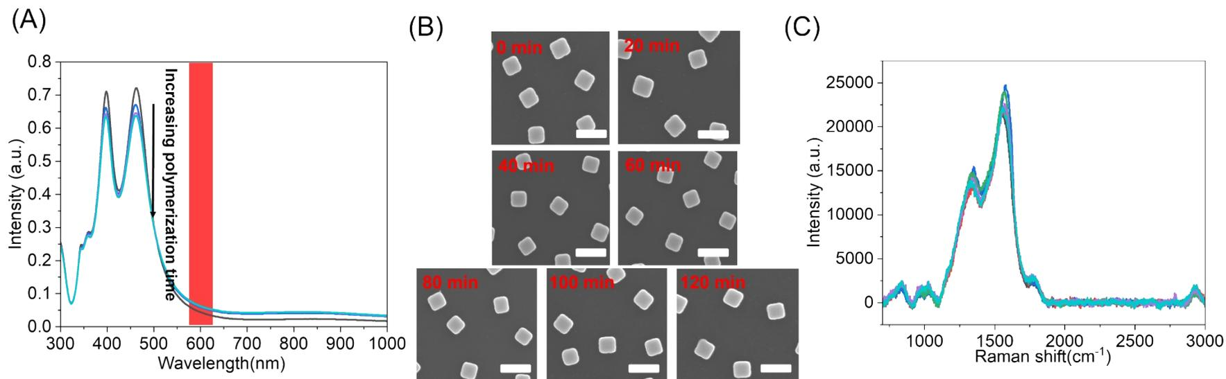
**Figure S19 Lactic acid polymerization of AgNC surface under  $600 \pm 20$  nm wavelength irradiation at  $-12$  °C.** (A) changes in the extinction spectrum of AgNC during polymerization process. (B) characterization of the morphology changes of AgNC during the polymerization process through SEM images. (C) changes in Raman spectra during the polymerization process were used to characterize the amount of polylactic acid formed on AgNC surface. The scale bar was 200 nm.
