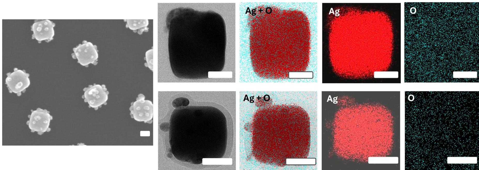
**Figure S3 Characterization of lactic acid polymerization on AgNC surface at 0 °C under irradiation by SEM, TEM, and EDX analysis.** The results showed that Ag oxidation on AgNC surface can be significantly inhibited compared with the reaction occurring at room temperature. The scale bar was 50 nm.
