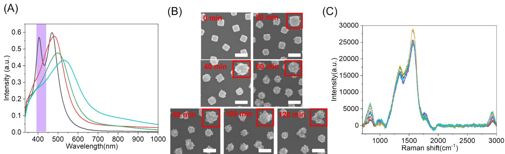
**Figure S7 Lactic acid polymerization of AgNC surface under  $420 \pm 20$  nm wavelength irradiation at room temperature.** (A) changes in the extinction spectrum of AgNC during polymerization process. (B) characterization of the morphology changes of AgNC during the polymerization process through SEM images. (C) changes in Raman spectra during the polymerization process were used to characterize the amount of polylactic acid formed on AgNC surface. The scale bar was 200 nm.
