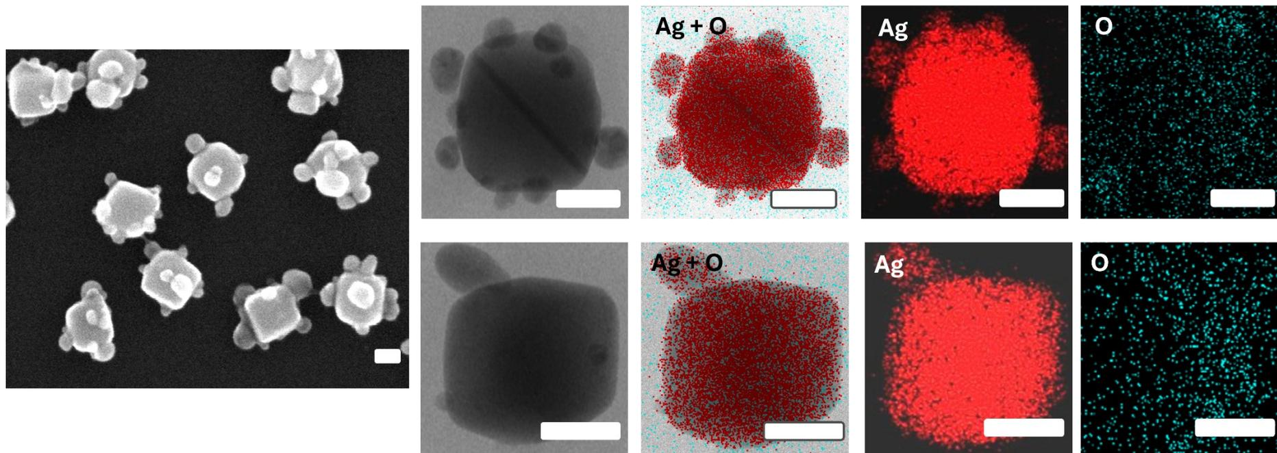
**Figure S1 Characterization of lactic acid polymerization on AgNC surface at room temperature under irradiation by SEM, TEM, and EDX analysis.** The results showed that in addition to the polymerization reaction, there was also oxidation of silver on AgNC surface. The scale bar was 50 nm.
