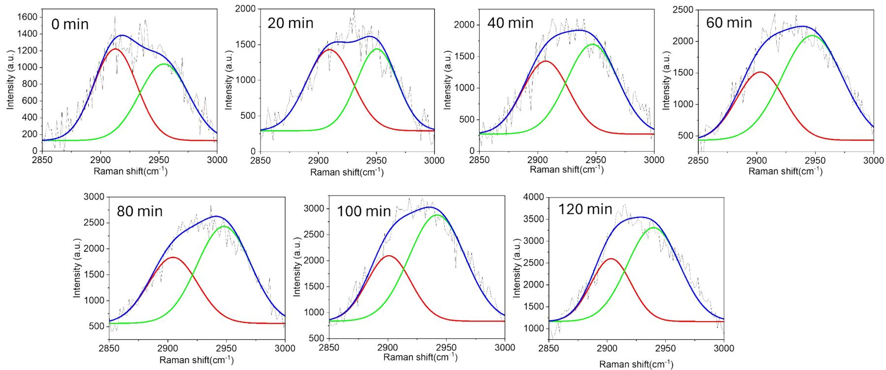
**Figure S10** The multi-curve fitting results of Raman scattering spectra during lactic acid polymerization on AgNC surface under  $420 \pm 20$  nm wavelength irradiation at  $0^\circ\text{C}$ . The results showed the multi-curve fitting at different polymerization times.
