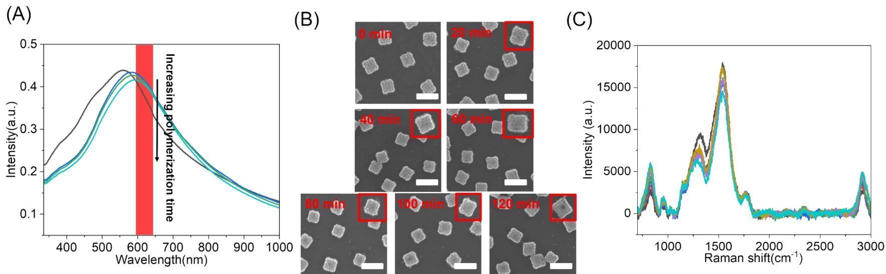
**Figure S25 Lactic acid polymerization of cage-like Au-AgNC surface under  $600 \pm 20$  nm wavelength irradiation at  $-12$  °C.** (A) changes in the extinction spectrum of AgNC during polymerization process. (B) characterization of the morphology changes of AgNC during the polymerization process through SEM images. (C) changes in Raman spectra during the polymerization process were used to characterize the amount of polylactic acid formed on AgNC surface. The scale bar was 200 nm.
