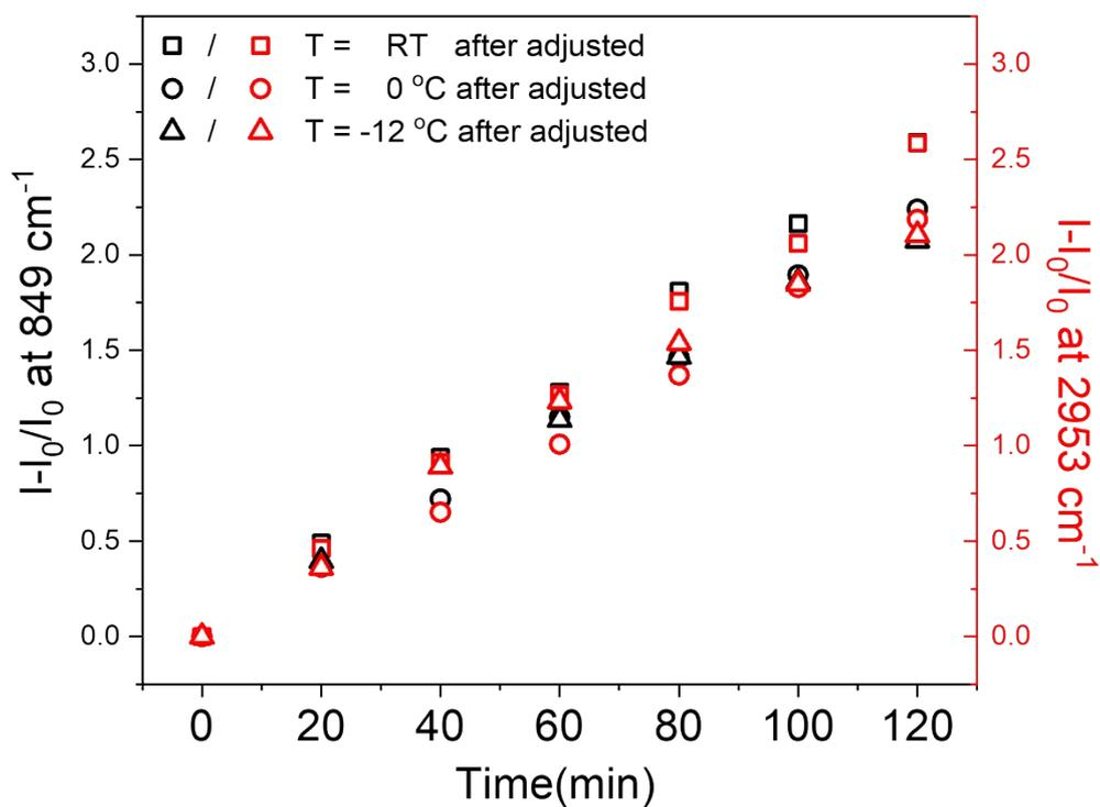
Figure S13 Changes in Raman scattering spectra during lactic acid polymerization on AgNC surface under  $420 \pm 20$  nm wavelength irradiation at -12 °C adjusted by the difference in the plasmon mode intensity of AgNC at 533 nm.
