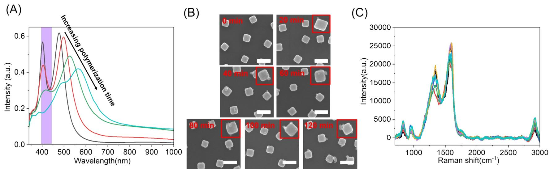
**Figure S11 Lactic acid polymerization of AgNC surface under  $420 \pm 20$  nm wavelength irradiation at  $-12$  °C.** (A) changes in the extinction spectrum of AgNC during polymerizing process. (B) characterization of the morphology changes of AgNC during the polymerization process through SEM images. (C) changes in Raman spectra during the polymerization process were used to characterize the amount of polylactic acid formed on AgNC surface. The scale bar was 200 nm.
