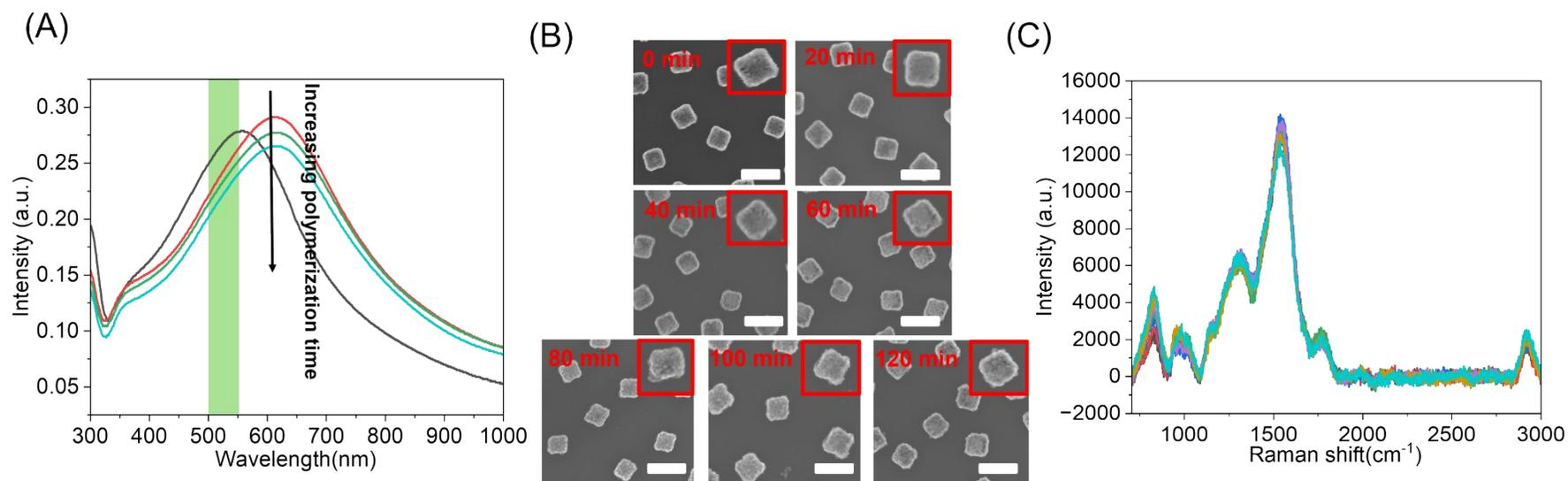
**Figure S23 Lactic acid polymerization of cage-like Au-AgNC surface under  $520 \pm 20$  nm wavelength irradiation at  $-12$  °C.** (A) changes in the extinction spectrum of AgNC during polymerization process. (B) characterization of the morphology changes of AgNC during the polymerization process through SEM images. (C) changes in Raman spectra during the polymerization process were used to characterize the amount of polylactic acid formed on AgNC surface. The scale bar was 200 nm.
