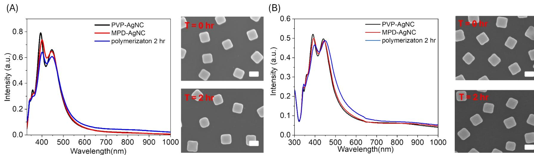
**Figure S2 Changes in optical properties of AgNC during lactic acid polymerization under reference reaction conditions. (A) at room temperature without irradiation. (B) at room temperature without a monomer.** Black curve: PVP coated AgNC. Red curve: MPD coated AgNC. Blue curve: AgNC after 2 hours of polymerization. And SEM images before and after 2 hours of polymerization showed that there was no lactic acid polymerization and Ag oxidation on the AgNC surface. The scale bar was 100 nm.
