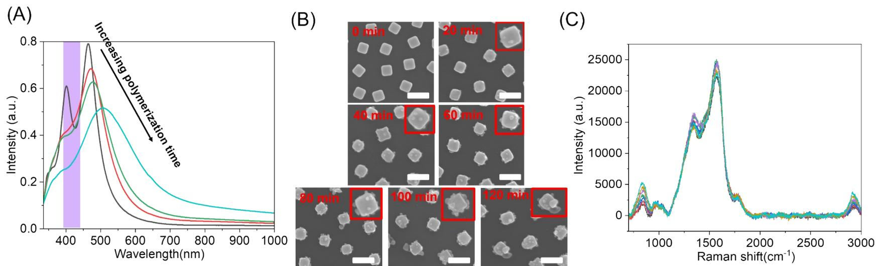
**Figure S9 Lactic acid polymerization of AgNC surface under  $420 \pm 20$  nm wavelength irradiation at 0 °C.** (A) changes in the extinction spectrum of AgNC during polymerization process. (B) characterization of the morphology changes of AgNC during the polymerization process through SEM images. (C) changes in Raman spectra during the polymerization process were used to characterize the amount of polylactic acid formed on AgNC surface. The scale bar was 200 nm.
