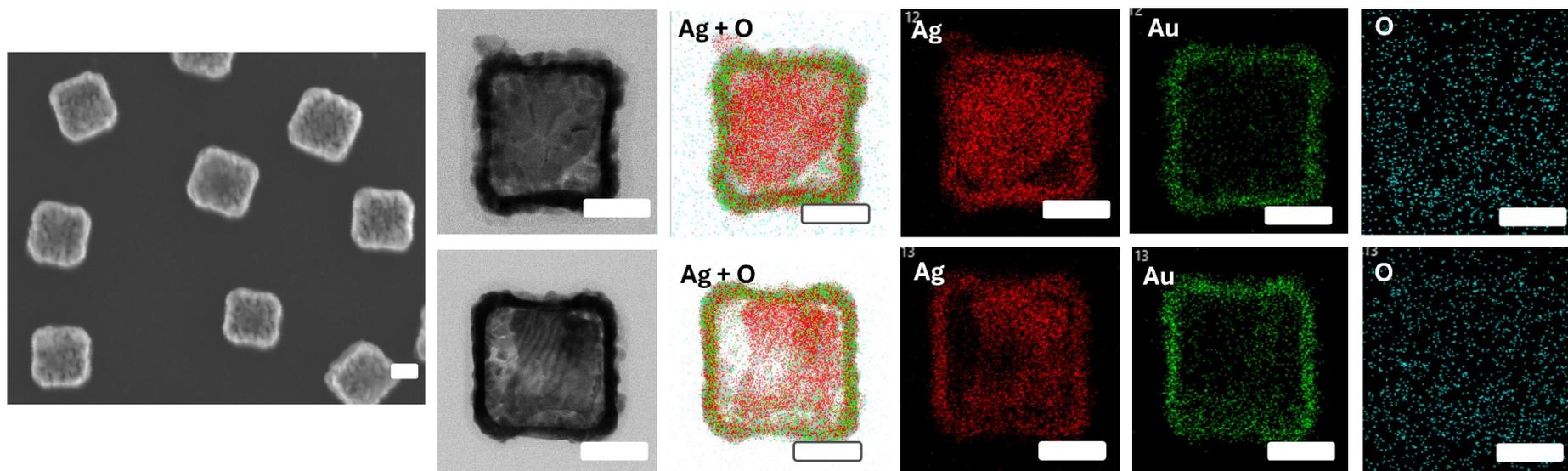
**Figure S15** Characterization of lactic acid polymerization on cage-like Au-AgNC surface at  $-12\text{ }^{\circ}\text{C}$  under irradiation by SEM, TEM, and EDX analysis. The results showed that Ag oxidation on cage-like Au-AgNC surface can be completely inhibited. The scale bar was 50 nm.
