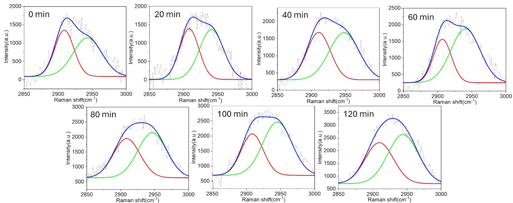
**Figure S28** The multi-curve fitting results of Raman scattering spectra during lactic acid polymerization on flower-like Au-AgNC surface under  $420 \pm 20$  nm wavelength irradiation at  $-12$  °C. The results showed the multi-curve fitting at different polymerization times.
