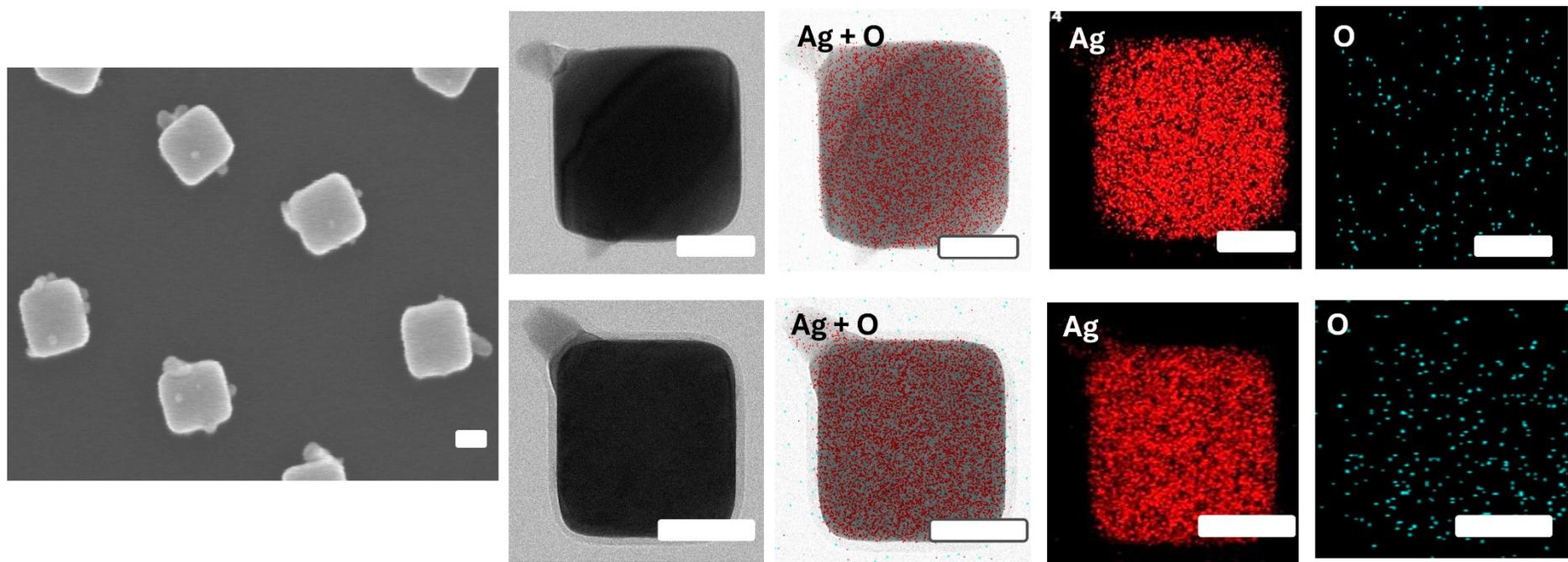
**Figure S4** Characterization of lactic acid polymerization on AgNC surface at -12 °C under irradiation by SEM, TEM, and EDX analysis. The results showed that Ag oxidation on AgNC surface can be completely inhibited. The scale bar was 50 nm.
