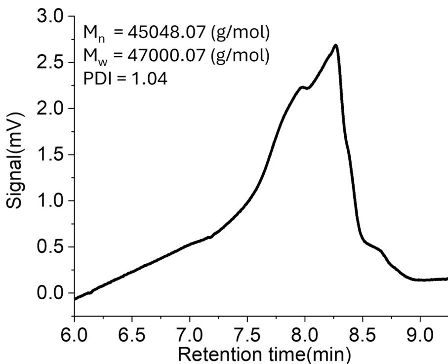
**Figure S14** The gel permeation chromatography (GPC) of poly(lactic acid) on the surface of AgNC at  $-12^{\circ}\text{C}$ . Poly(lactic acid) molecules can be removed from the surface of nanocrystals by ultrasonic treatment, and then the molecular weight of poly(lactic acid) can be measured by gel permeation chromatography (GPC). The results showed  $M_n \sim 45000$  g/mole,  $M_w \sim 47000$ , and PDI  $\sim 1.04$ .
