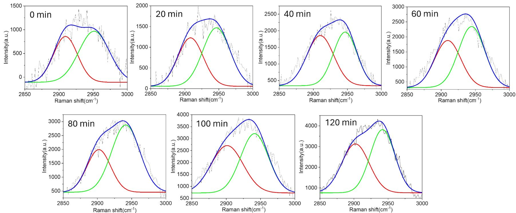
**Figure S8** The multi-curve fitting results of Raman scattering spectra during lactic acid polymerization on AgNC surface under  $420 \pm 20$  nm wavelength irradiation at room temperature. The results showed the multi-curve fitting at different polymerization times.
