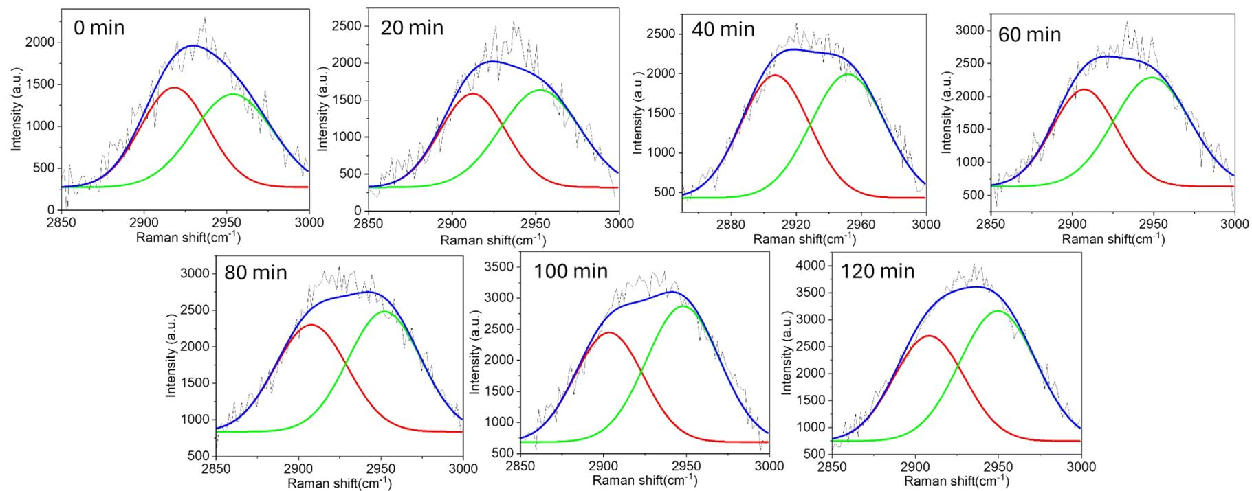
**Figure S32** The multi-curve fitting results of Raman scattering spectra during lactic acid polymerization on flower-like Au-AgNC surface under  $600 \pm 20$  nm wavelength irradiation at  $-12$  °C. The results showed the multi-curve fitting at different polymerization times.
