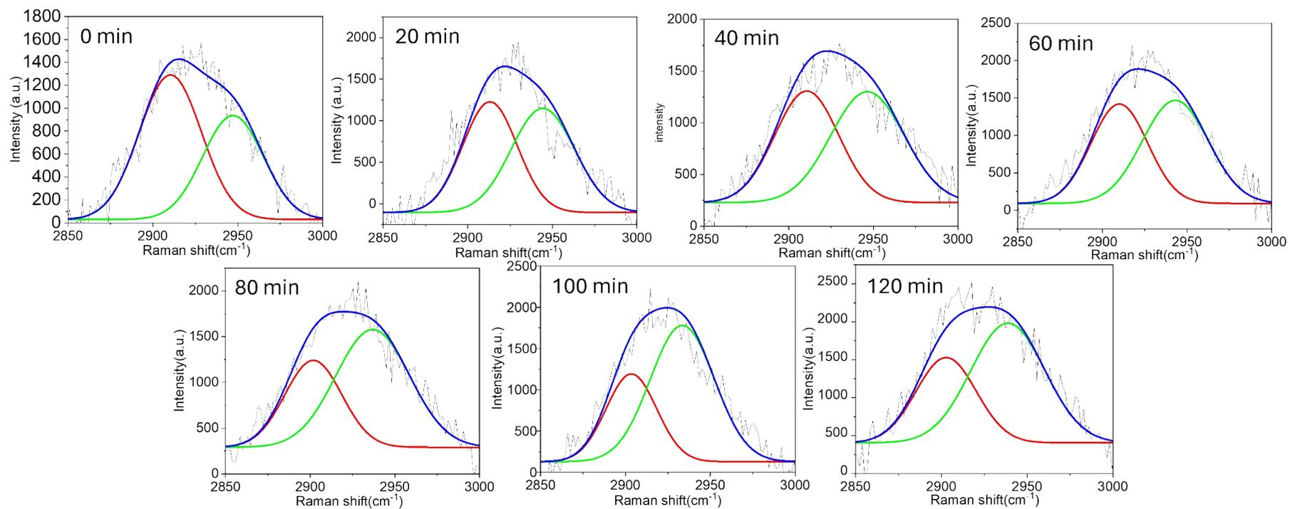
**Figure S24** The multi-curve fitting results of Raman scattering spectra during lactic acid polymerization on cage-like Au-AgNC surface under  $520 \pm 20$  nm wavelength irradiation at  $-12$  °C. The results showed the multi-curve fitting at different polymerization times.
