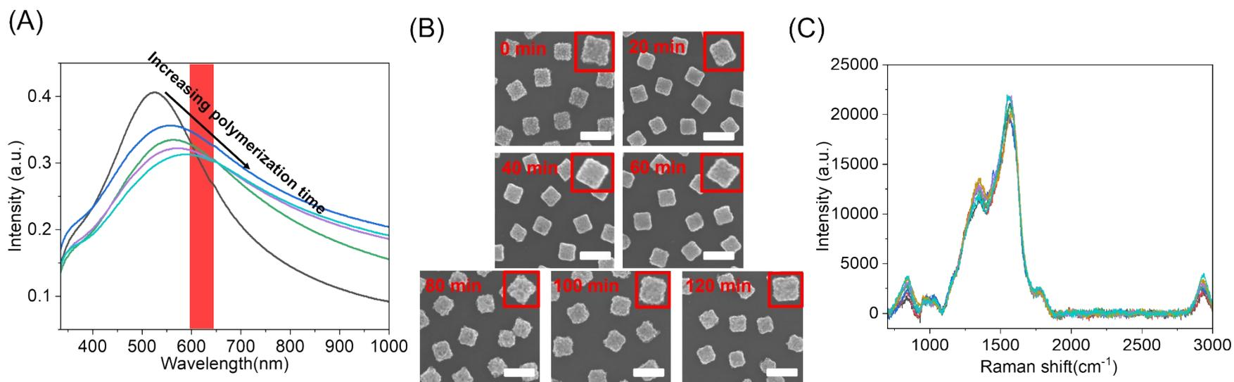
**Figure S31 Lactic acid polymerization of flower-like Au-AgNC surface under  $600 \pm 20$  nm wavelength irradiation at  $-12$  °C.** (A) changes in the extinction spectrum of AgNC during polymerization process. (B) characterization of the morphology changes of AgNC during the polymerization process through SEM images. (C) changes in Raman spectra during the polymerization process were used to characterize the amount of poly(lactic acid) formed on AgNC surface. The scale bar was 200 nm.
