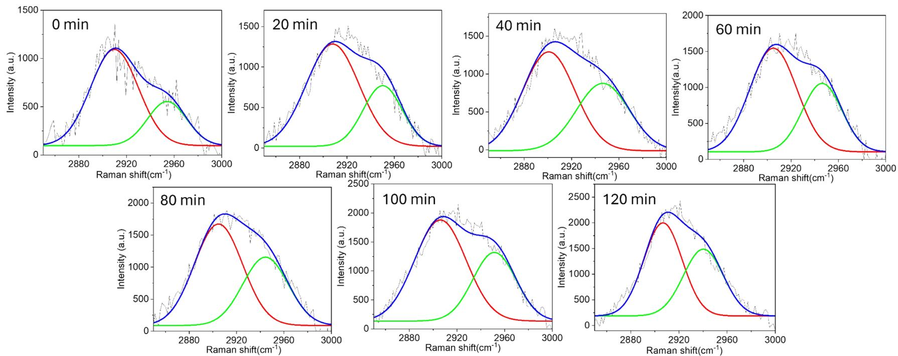
**Figure S30** The multi-curve fitting results of Raman scattering spectra during lactic acid polymerization on flower-like Au-AgNC surface under  $520 \pm 20$  nm wavelength irradiation at  $-12$  °C. The results showed the multi-curve fitting at different polymerization times.
