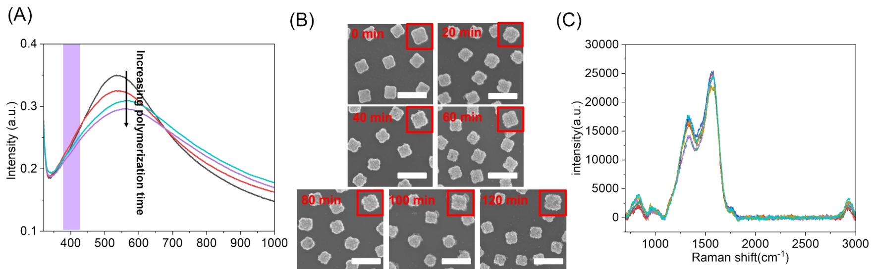
**Figure S27 Lactic acid polymerization of flower-like Au-AgNC surface under  $420 \pm 20$  nm wavelength irradiation at  $-12$  °C.** (A) changes in the extinction spectrum of AgNC during polymerization process. (B) characterization of the morphology changes of AgNC during the polymerization process through SEM images. (C) changes in Raman spectra during the polymerization process were used to characterize the amount of polylactic acid formed on AgNC surface. The scale bar was 200 nm.
