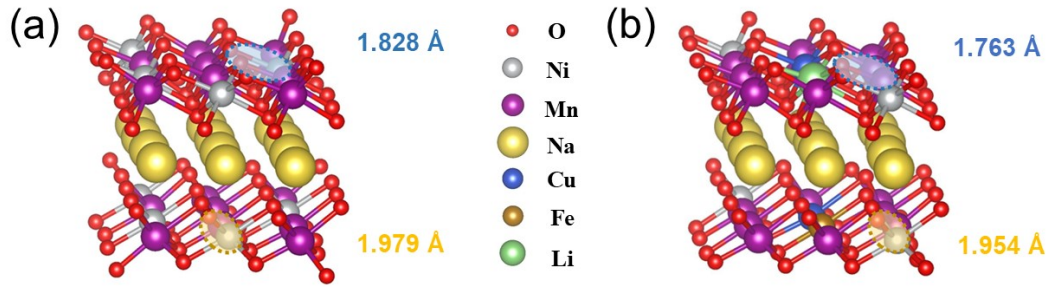
Fig. S1. The optimized structures of (a) NMNO and (b) NMNCLFO based on the density functional theory (DFT) calculation. The DFT calculations were carried out using the Vienna Ab-initio Simulation Package (VASP) with the frozen-core all-electron projector-augment-wave (PAW) method. The Perdew-Burke-Ernzerhof (PBE) of generalized gradient approximation (GGA) was adopted to describe the exchange and correlation potential. The cutoff energy for the plane-wave basis set was set to 450 eV. A 2-layer 2 \times 3 \text{Na}_{0.7}\text{Mn}_{0.65}\text{Ni}_{0.35}\text{O}_2(001) supercell (NMNO) was used. The vacuum region of 20 Å above them were added to ensure the decoupling between neighboring systems. Four Ni atoms in NMNO were randomly replaced with two Cu atom, one Li and one Fe atoms to simulate the model of \text{Na}_{0.7}\text{Mn}_{0.65}\text{Ni}_{0.15}\text{Cu}_{0.12}\text{Li}_{0.03}\text{Fe}_{0.05}\text{O}_2 (NMNCLFO). The geometry optimizations were performed until the forces on each ion was reduced below 0.01 eV/Å, and a 1 \times 1 \times 1 Gamma k-point sampling of the Brillouin zone was used. The van der Waals (vdW) interactions have been considered by using DFT-D3 method of Grimme.
