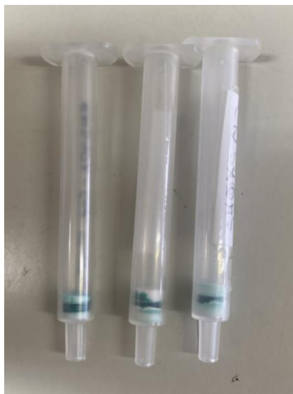
Figure S5. Image of the capture device incorporating SPE cartridges.
