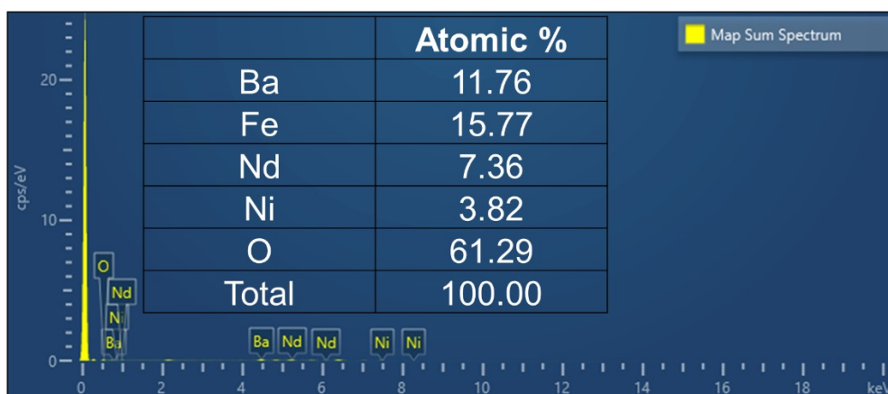
Figure S4 SEM-EDS results showing elements composition of NBFN.
