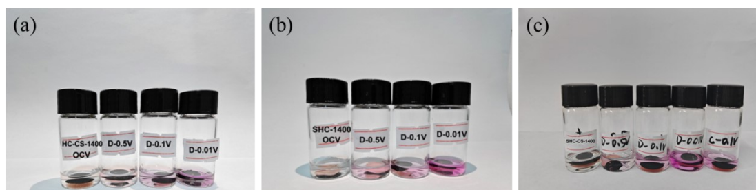
Figure S20 Optical photographs of (a) HC-CS-1400, (b) SHC-1400 and (c) SHC-CS-1400 electrodes immersed in an ethanol solution containing phenolphthalein at different discharge stages
