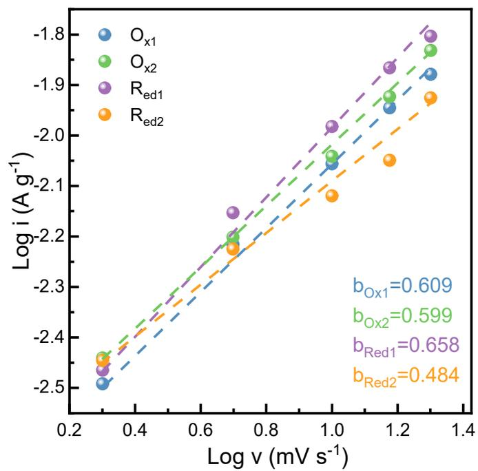
Figure S10. The relationship between peak current and scan rate in the logarithm ( $\text{MnO}_2$ ).
