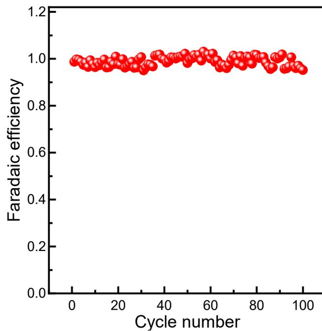
**Figure S17.** The effluent Faradaic efficiency for the FLA-MnO<sub>2</sub>||AC cell during 100 cycles.
