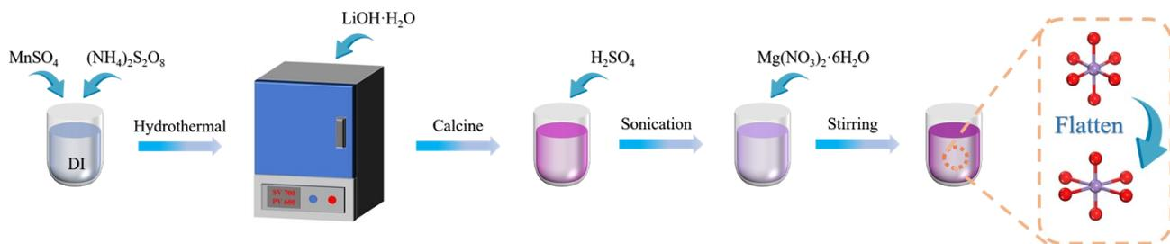
**Figure S1.** Illustration of the synthesis of FLA-MnO<sub>2</sub>.
