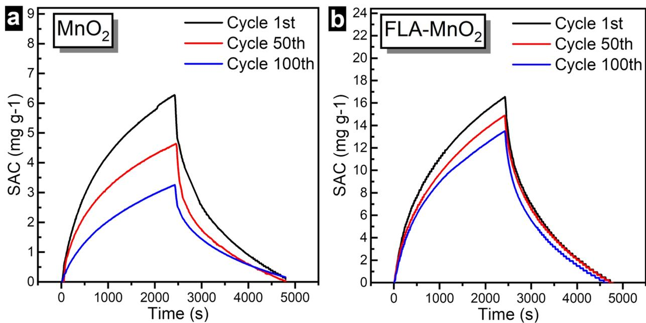
Figure S16. Electroadsorption/desorption kinetics of (a) MnO<sub>2</sub>, (b) FLA-MnO<sub>2</sub> at the Cycle 1st, 50th and 100th.
