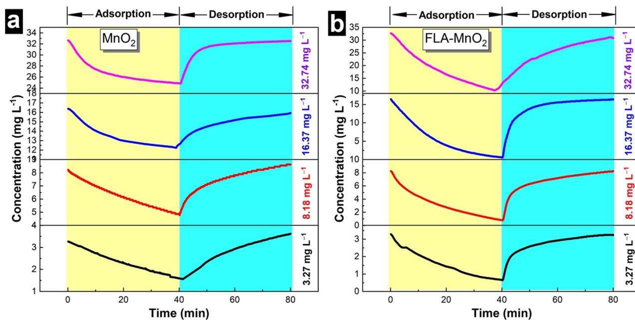
Figure S13. Plots of concentration versus time in HCDI cell with the  $\text{MnO}_2$  and FLA- $\text{MnO}_2$  electrode at 1.2 V with varying feed concentrations.
