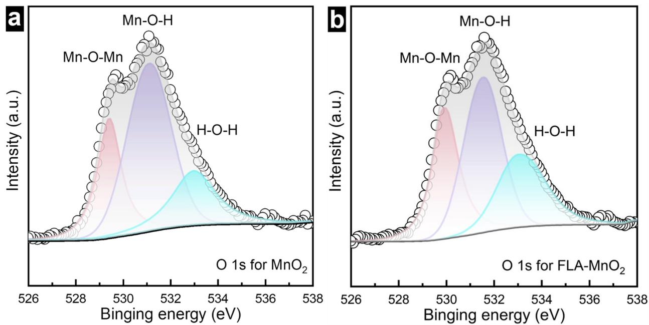
**Figure S6.** O 1s survey of (a) MnO<sub>2</sub>, (b) FLA-MnO<sub>2</sub>.
