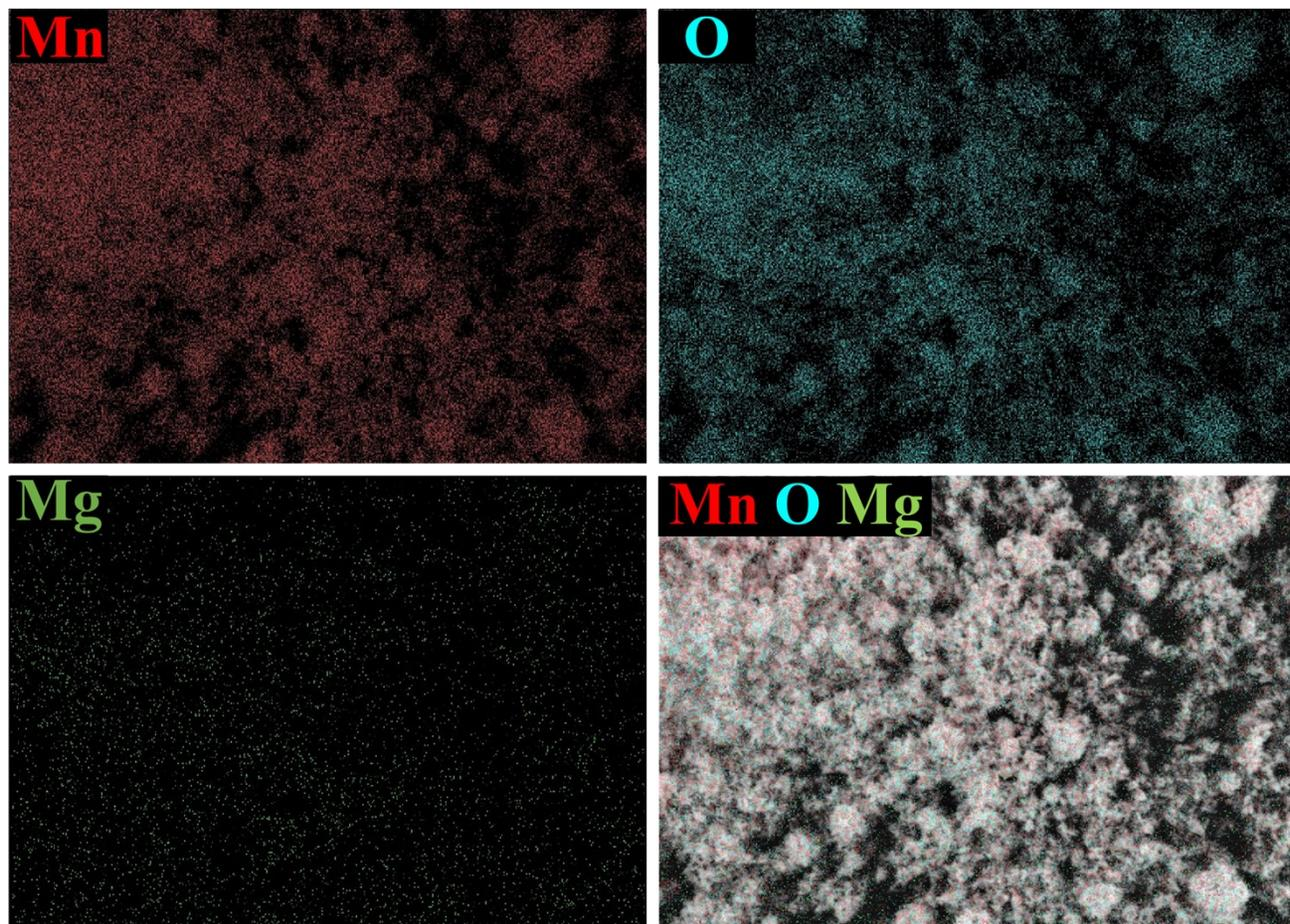
Figure S4. Element mapping of FLA-MnO<sub>2</sub>.
