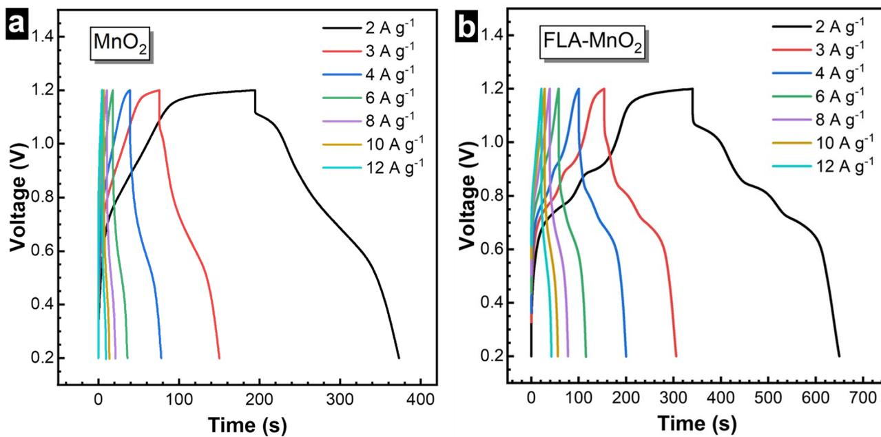
**Figure S7.** GCD curves of  $\text{MnO}_2$  and  $\text{FLA-MnO}_2$  electrodes at different specific currents: (a)  $\text{MnO}_2$ , (b)  $\text{FLA-MnO}_2$ ,
