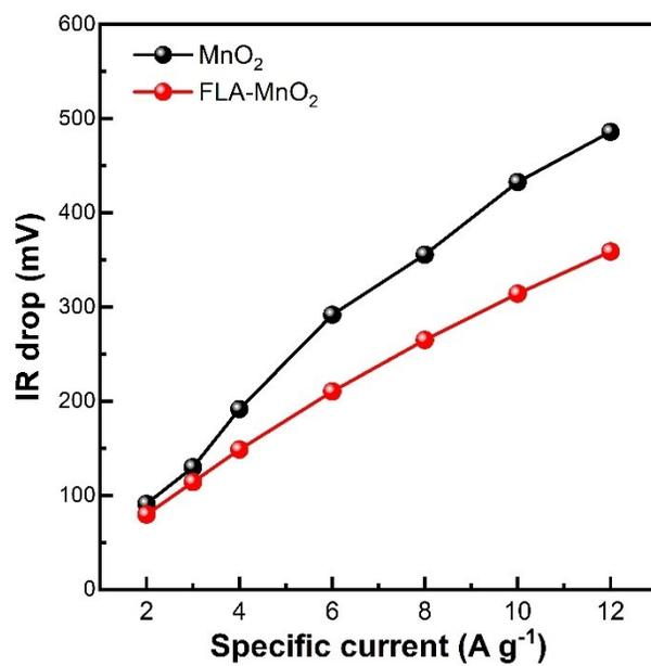
**Figure S9.** IR drop measured by the discharge curves at different specific currents.
