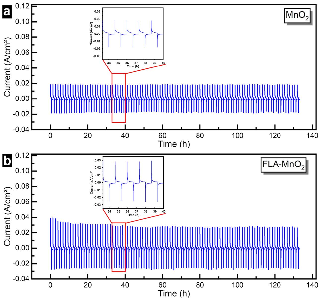
Figure S15. The current profile during 100-time adsorption-desorption cycling test of (a) MnO<sub>2</sub>, (b) FLA-MnO<sub>2</sub>.
