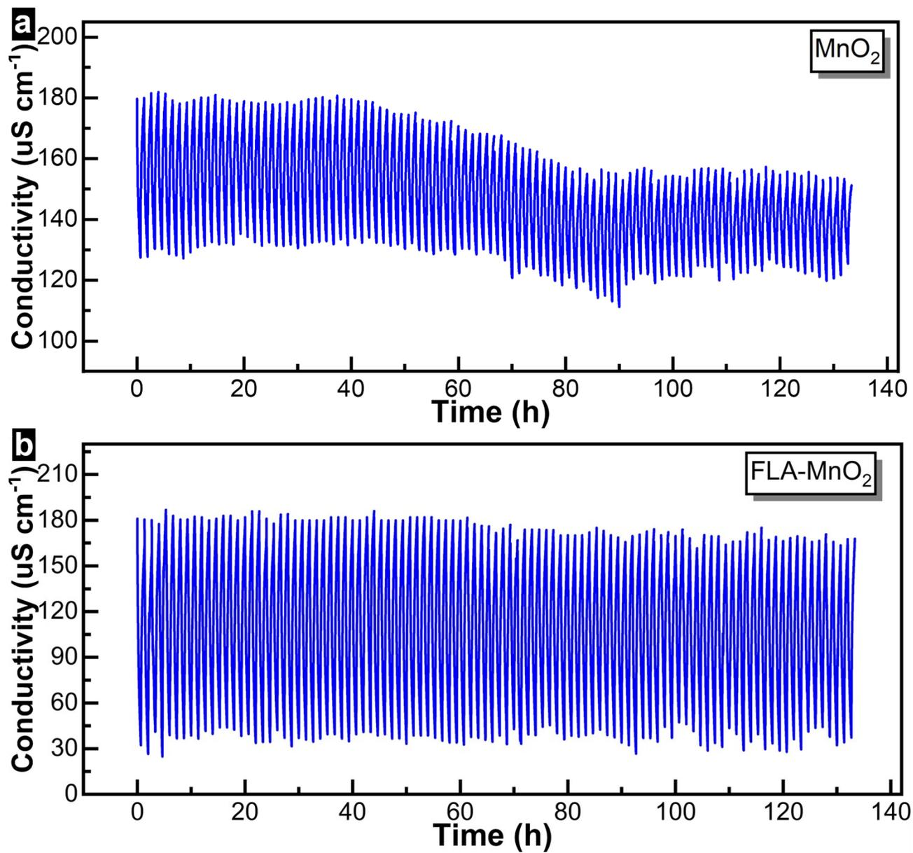
Figure S14. Conductivity curve during 100-time adsorption-desorption cycling test of (a)  $\text{MnO}_2$ , (b) FLA- $\text{MnO}_2$ .
