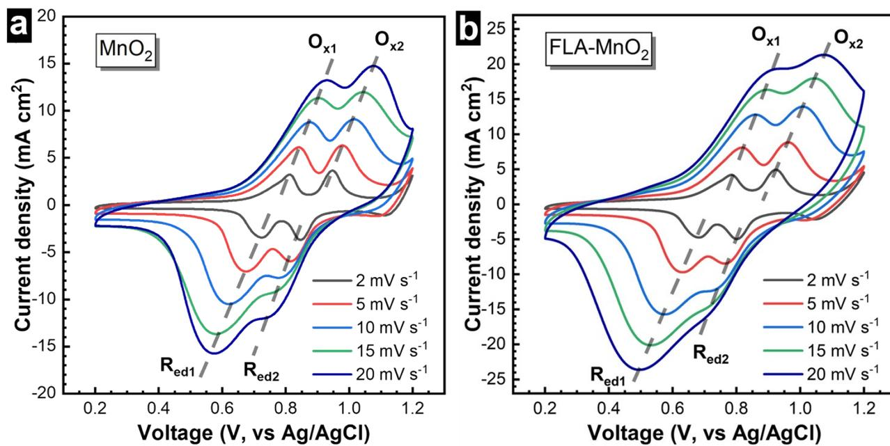
Figure S8. CV curves of MnO<sub>2</sub> and FLA-MnO<sub>2</sub> electrodes at different specific currents: (a) MnO<sub>2</sub>, (b) FLA-MnO<sub>2</sub>,
