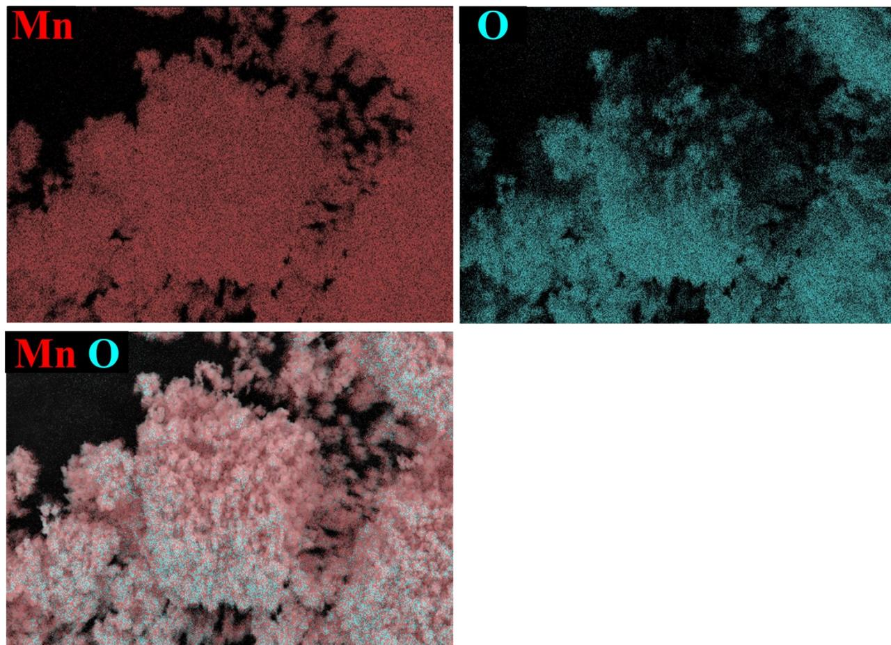
Figure S3. Element mapping of MnO<sub>2</sub>.
