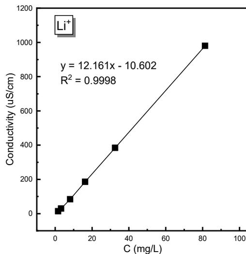
**Figure S18.** The correlation between the solutions with different  $\text{Li}^+$  concentrations prepared in the laboratory and the conductivity values obtained.
