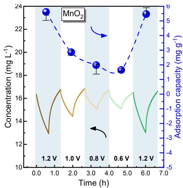
**Figure S12.** Plots of concentration versus time in HC DI cell with the MnO<sub>2</sub> electrode in 16.37 mg L<sup>-1</sup> Li<sup>+</sup> ion solution at varying cell voltages and plots of adsorption capacity versus cell voltage (line with symbols).
