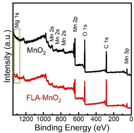
**Figure S5.** XPS survey of MnO<sub>2</sub> and FLA-MnO<sub>2</sub>.
