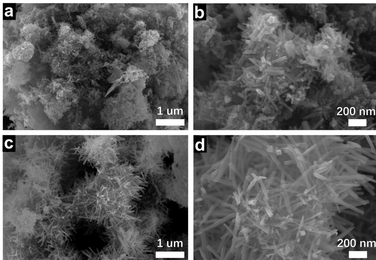
**Figure S2.** SEM images of (a, b) MnO<sub>2</sub>, (c, d) FLA-MnO<sub>2</sub>.
