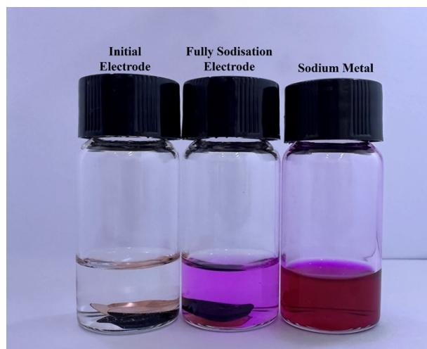
**Fig. S19.** Color changes of the reference samples reacting with a 1% phenolphthalein ethanol solution: The samples from left to right are the original HCSNP electrode, the fully discharged HCSNP electrode, and metallic sodium.
