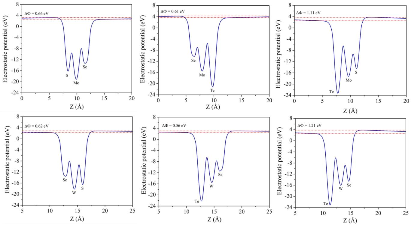
SFig. 2 The electrostatic potential of the Janus structures, MoSSe, MoSeTe, MoSTe, WSSe, WSeTe and WSTe. The red-colored dashed lines indicate the vacuum levels corresponding to the two sides of the Janus SLs.
