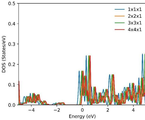
SFig. 4: The contribution of the H atom 1s orbital density of states (DOS) in the MoS<sub>2</sub> SL under four distinct coverage ratios.
