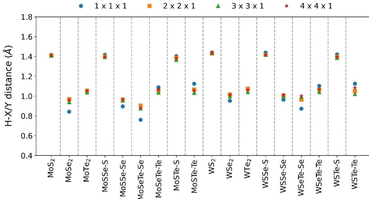
SFig. 6 The vertical H-X/Y distances between the adsorbed H atom and the surface of adsorption in all the considered regular and Janus TMDs. The energetically favorable sites are chosen for the study i.e., C-site for S surfaces and M-site for Se and Te surfaces.
