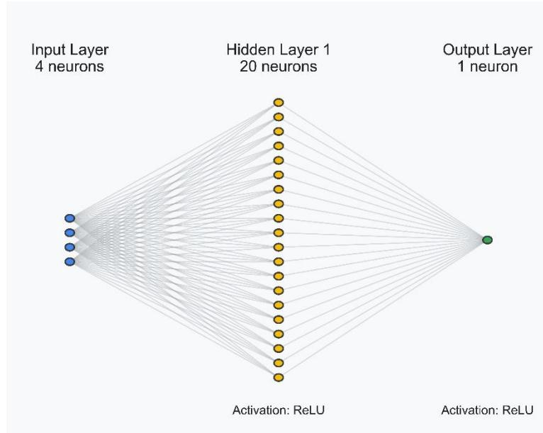
SFig. 8: The schematic of the feedforward neural network with an input layer, one hidden layer, and an output layer.
