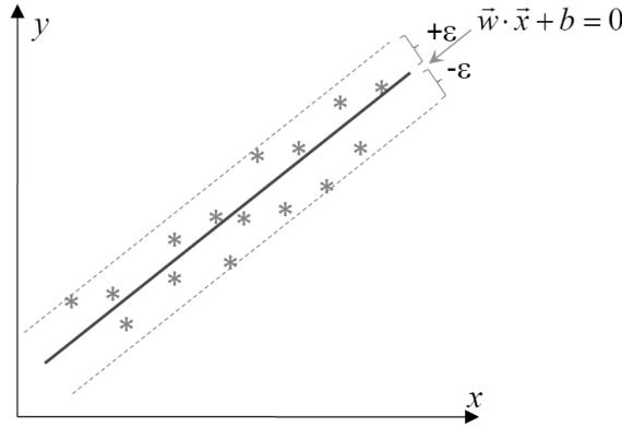
SFig. 7 Illustration of SVR in 2D-plane. Here,  $\bar{x}$  denotes a point,  $(x, y)$  and  $\bar{w} = (w_1, w_2)$  denotes the corresponding coefficients. Regression line:  $\bar{w} \cdot \bar{x} + b = w_1x + w_2y + b = 0$ .
