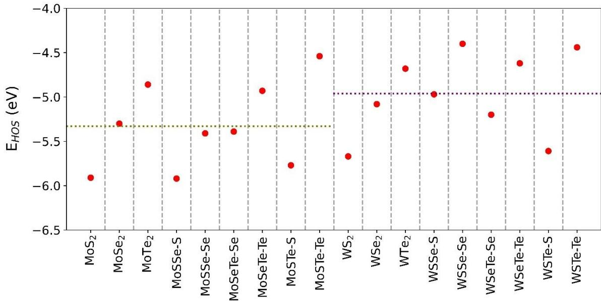
SFig. 3 The variation of the highest occupied state,  $E_{HOS}$  of various TMD SLs. The olive and purple-colored dotted lines indicate the average  $E_{HOS}$  values of the Mo and W based TMDs.
