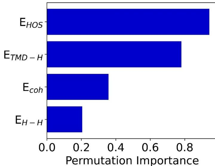
SFig. 9 The importance of each descriptor in predicting the H atom adsorption energy  $E_{ads}$  on the TMD surfaces with the MLPR model.
