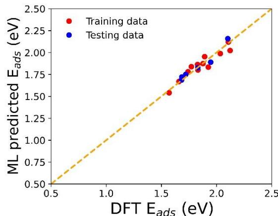
SFig. 10. The DFT calculated verses ML predicted  $E_{ads}$  with the linear regression model by considering only the regular TMDs.
