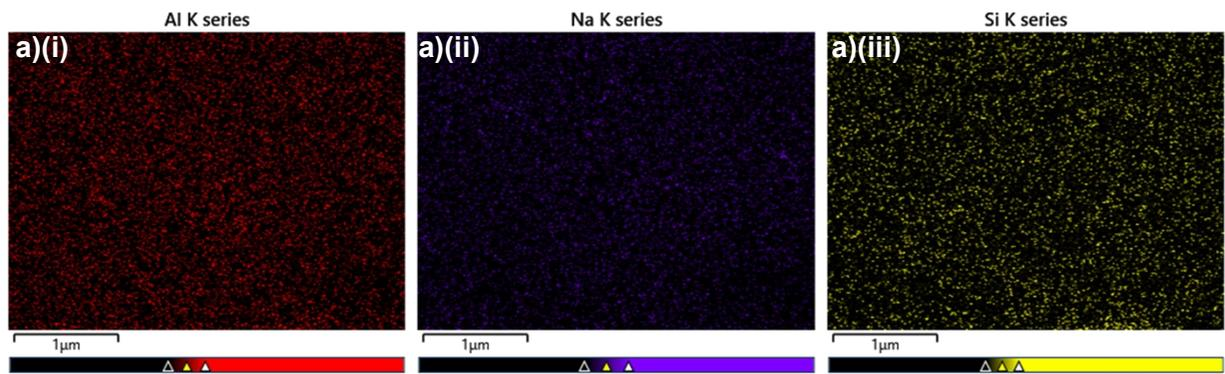
**Figure. S3** FE-SEM (a)(i-iii) elemental mapping images of ZMO@C composite
