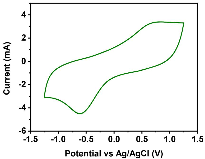
**Figure. S4** CV measurements using a three-electrode cell tested in 1 M LCP/ACN electrolyte at the scan rate of 25 mV/s in the potential window between -1.25 to 1.25 V
