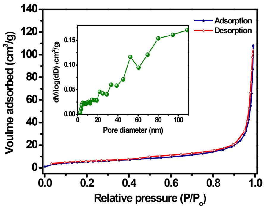
**Figure. S2** Nitrogen adsorption-desorption isotherms, and inset BJH pore volume curve of ZMO@C composite
