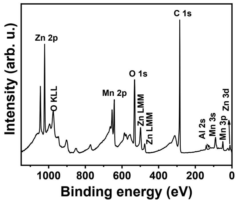
**Figure. S1** XPS survey spectrum of ZMO@C composite
