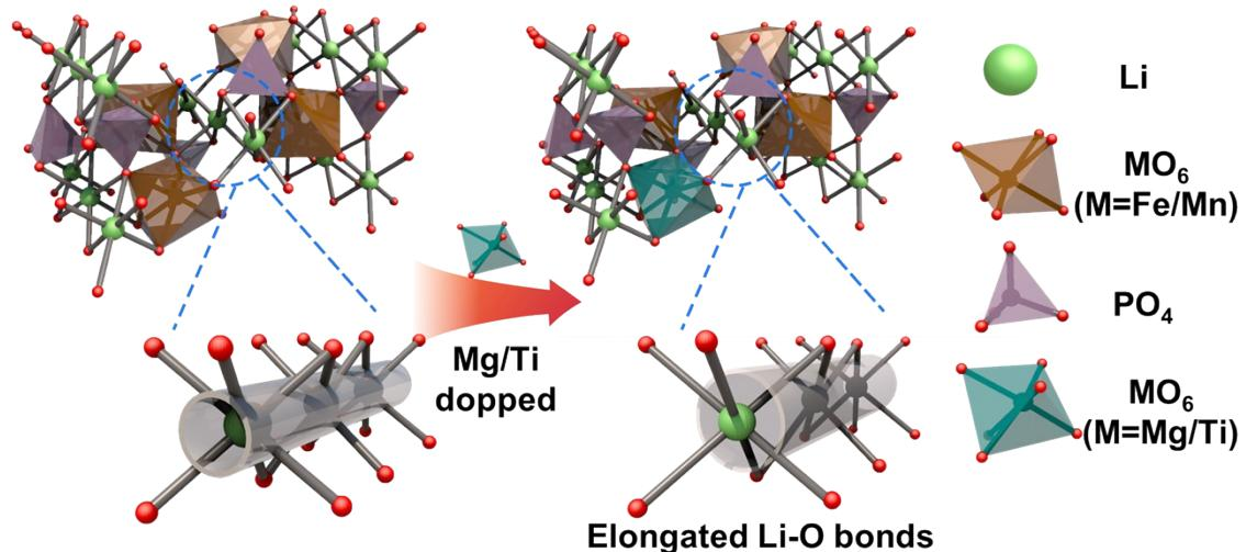
**Fig. S4** The structural diagram of the elongation of the Li-O bonds.
