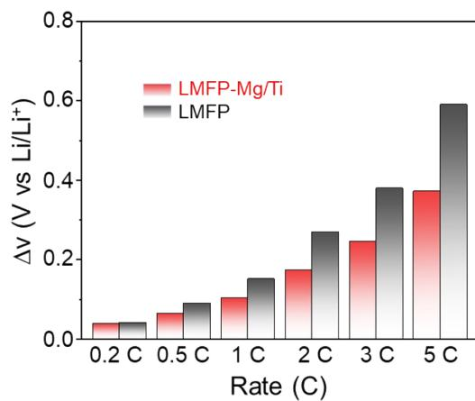
**Fig. S8** Overpotential of Mn plateau for LFMP and LMFP-Mg/Ti at different current rates.
