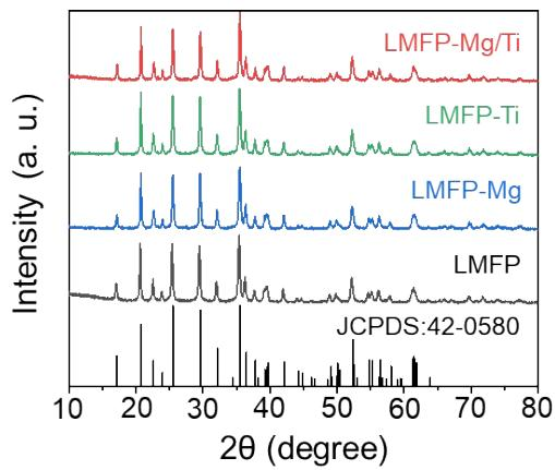
**Fig. S1** XRD patterns of LMFP, LMFP-Mg, LMFP-Ti, and LMFP-Mg/Ti.
