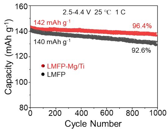
**Fig. S9** The cycle performance of LMFP and LMFP-Mg/Ti at 1 C.
