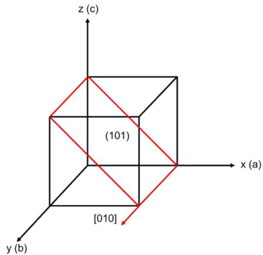
**Fig. S5** The schematic of crystal plane.
