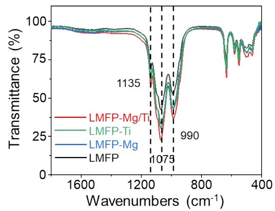
**Fig. S6** The FT-IR spectroscopy of LMFP, LMFP-Mg, LMFP-Ti and LMFP-Mg/Ti.
