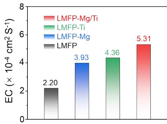
**Fig. S14** Electronic conductivity of the LMFP, LMFP-Mg, LMFP-Ti and LMFP-Mg/Ti.
