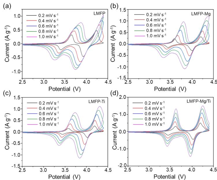
**Fig. S13** CV curves of (a) LMFP, (b) LMFP-Mg, (c) LMFP-Ti, and (d) LMFP-Mg/Ti at various sweep rates from  $0.2$  to  $1.0 \text{ mV}\cdot\text{s}^{-1}$  in  $2.5$ - $4.4$  V.
