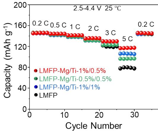
**Fig. S11** The rate performance of cathode with different  $Mg^{2+}$  and  $Ti^{4+}$  contents.
