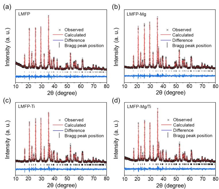
**Fig. S2** XRD refinement results of LMFP, LMFP-Mg, LMFP-Ti, and LMFP-Mg/Ti.
