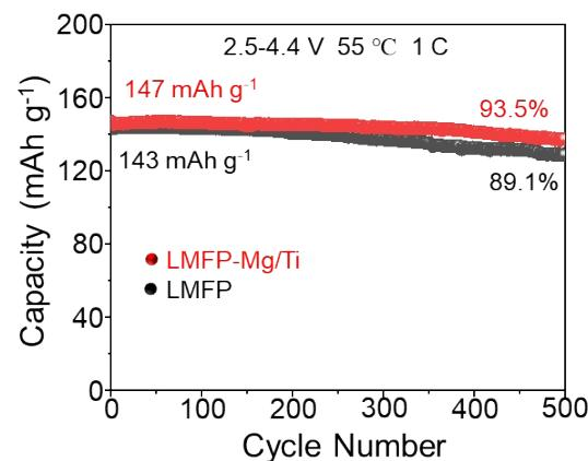
**Fig. S10** The cycle performance of LMFP and LMFP-Mg/Ti at 55 °C.
