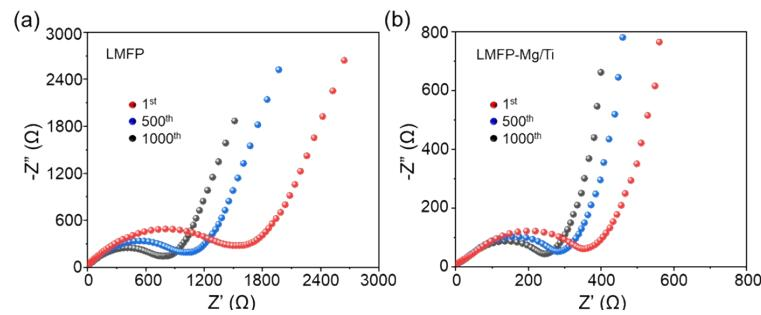
**Fig. S15** Nyquist curves of (a) LMFP and (b) LMFP-Mg/Ti before and after cycling.
