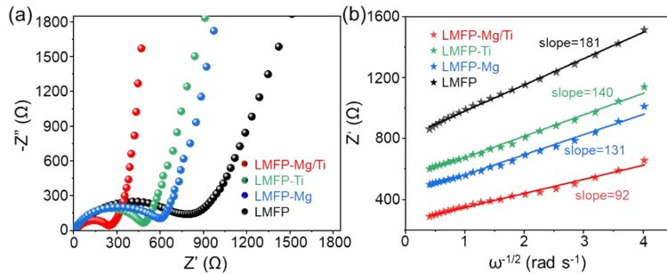
**Fig. S12** The linear relationship of  $Z'$  versus  $\omega^{-1/2}$  in the low-frequency region for LFMP, LMFP-Mg, LMFP-Ti, and LMFP-Mg/Ti.
