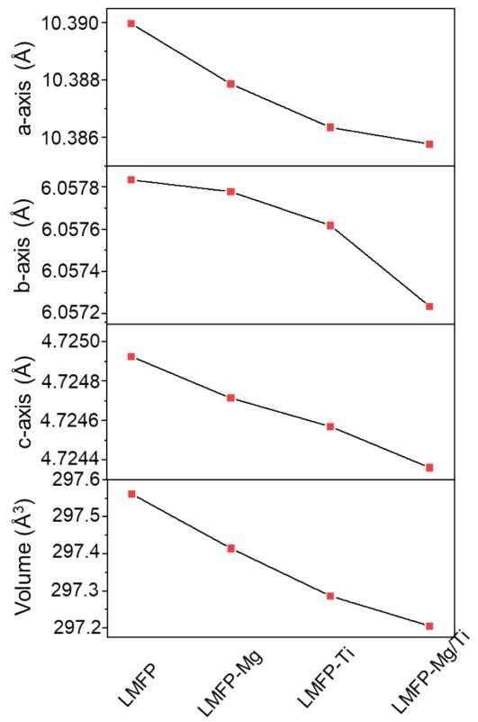
**Fig. S3** Refined cell parameters of both a, b, c, and v for LMFP, LMFP-Mg, LMFP-Ti, and LMFP-Mg/Ti.
