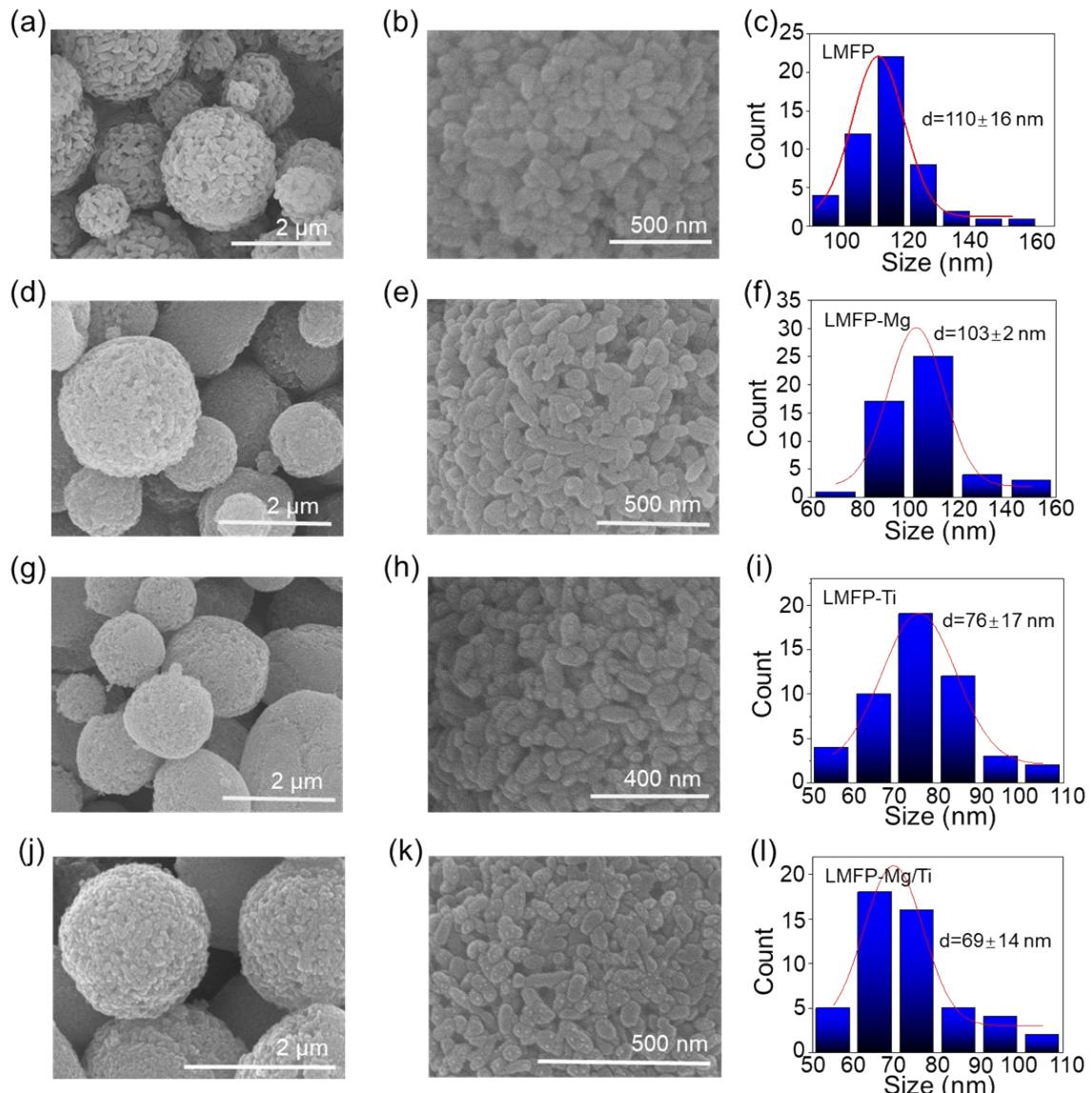
**Fig. S7** The SEM images of (a, b, c) LMFP, (d, e, f) LMFP-Mg, (g, h, i) LMFP-Ti, and (j, k, l) LMFP-Mg/Ti at different resolutions and their particle size analysis.
