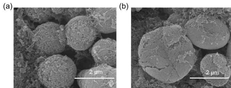
**Fig. S16** SEM images of (a) LMFP-Mg/Ti and (b) LMFP after 1000 cycles at 3 C.
